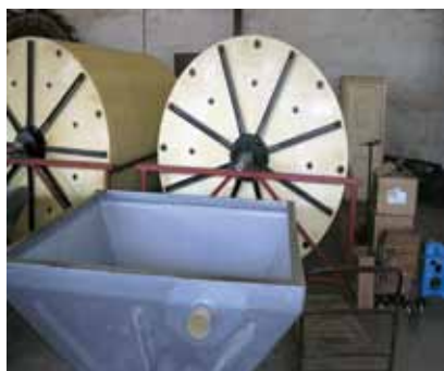
Components of a rotating bio-contactor
