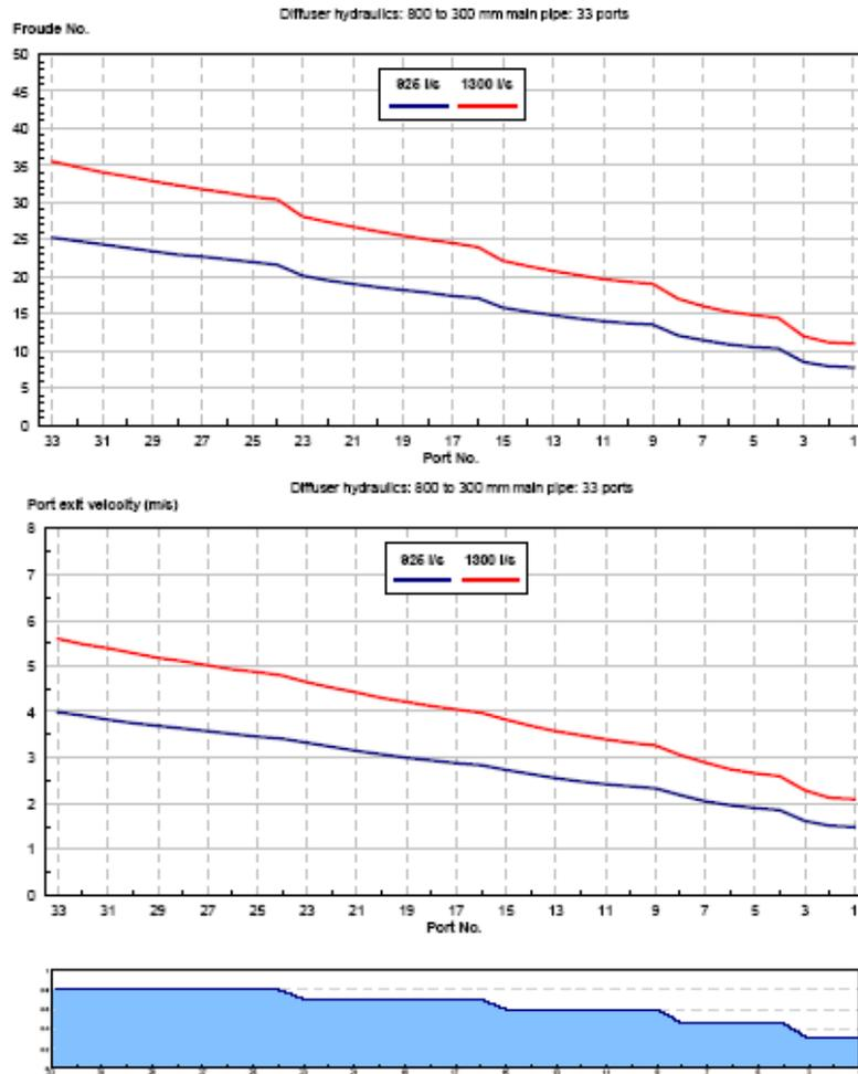
FIGURE 6.35 b: Example of graphical output required to evaluate hydraulic functionality: Port Froude Numbers (top) and port exit velocities (bottom)
