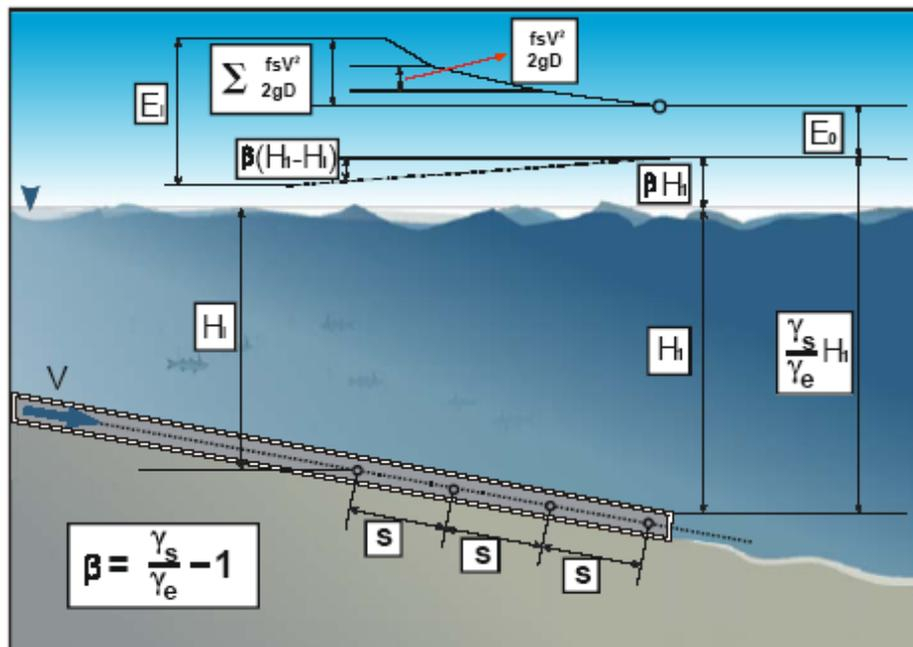
FIGURE 6.33: Head losses in a multi-port diffuser (Williams, 1985)
