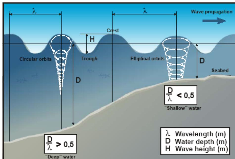
FIGURE 6.5: Description of a wave
