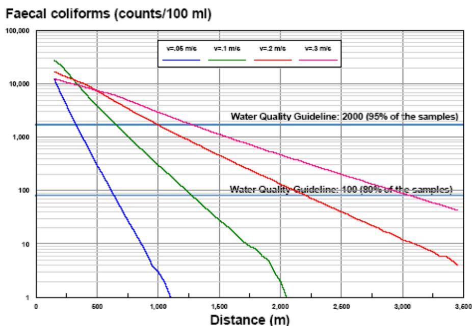
**FIGURE 6.55:** Example: Variation in distance from the discharge location at which faecal coliform counts comply with environmental quality objectives (or water quality guidelines) under a range of current velocities
