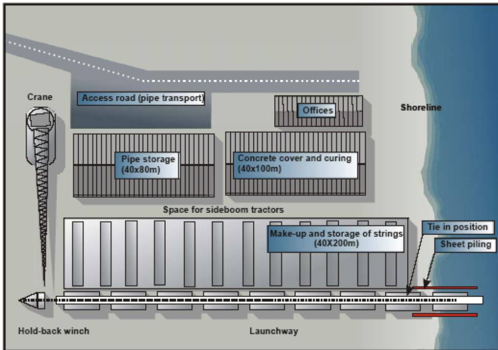
FIGURE 6.56: A typical construction-launching site for the bottom-pull method
