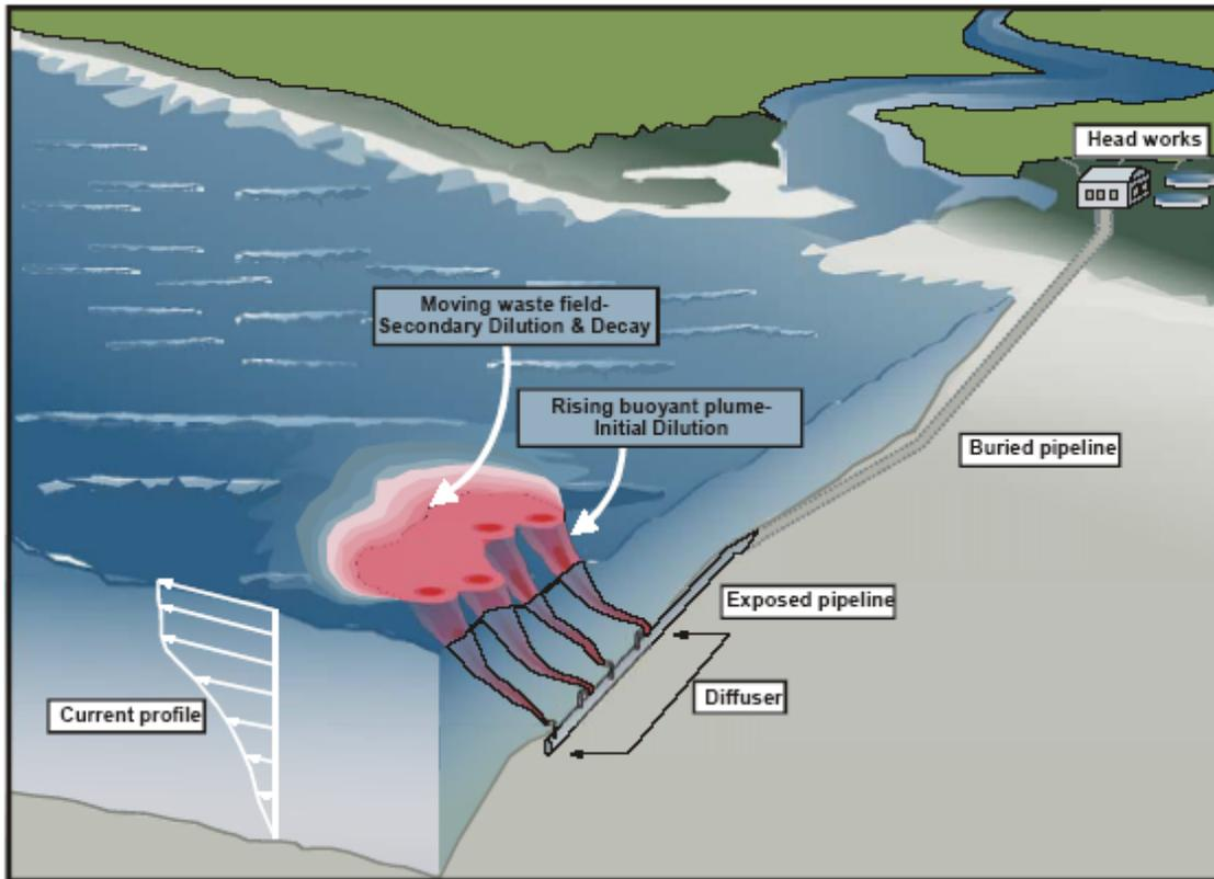
**FIGURE 6.36:** *Illustration of the different dilution components making up the total achievable dilution for an offshore marine outfall*
