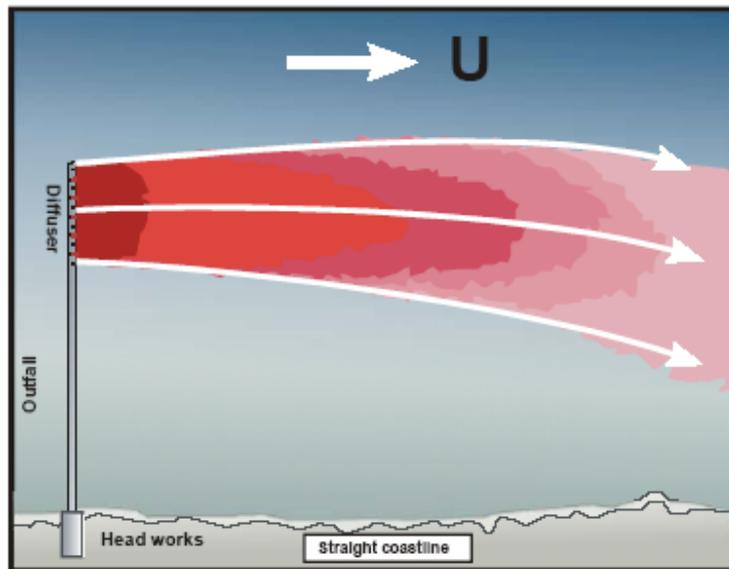
FIGURE 6.42: Illustration of a waste field along a straight coastline using Brooks's surface plume model
