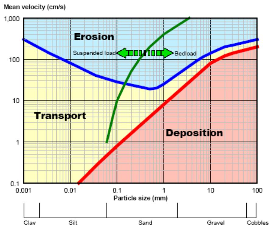
**FIGURE 6.53:** *The effect of current velocities on the erosion, transport and deposition of sediments (Gunnerson, 1988)*
