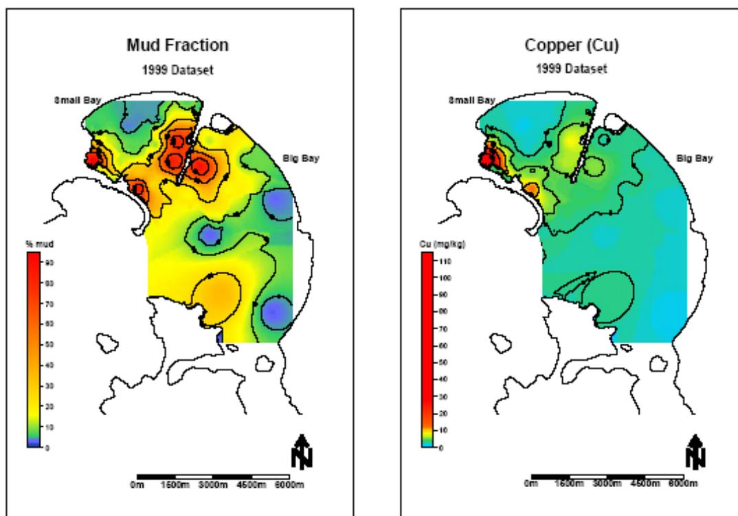
**FIGURE 6.54: Plot of the distribution of copper and particle size in Saldanha Bay (South Africa), showing the strong correlation between depositional areas and trace metals deposition**
