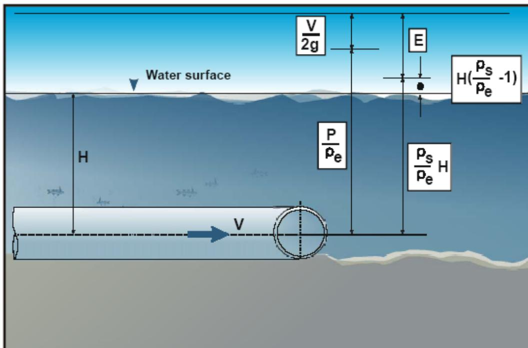
FIGURE 6.32: Energy balance for flow from a single port
