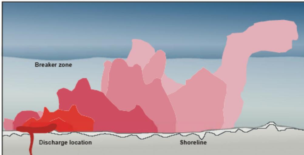
**FIGURE 6.46:** Example of a dye dispersion test during a continuous release to the surf zone in False Bay (Cape Town)
