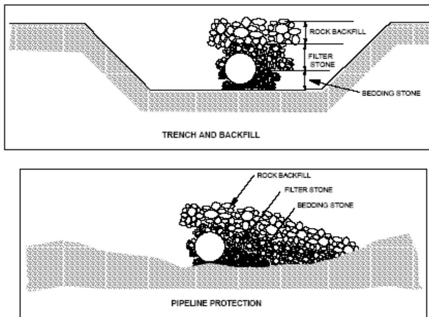
FIGURE 6.57: Examples of backfill cross-sections
