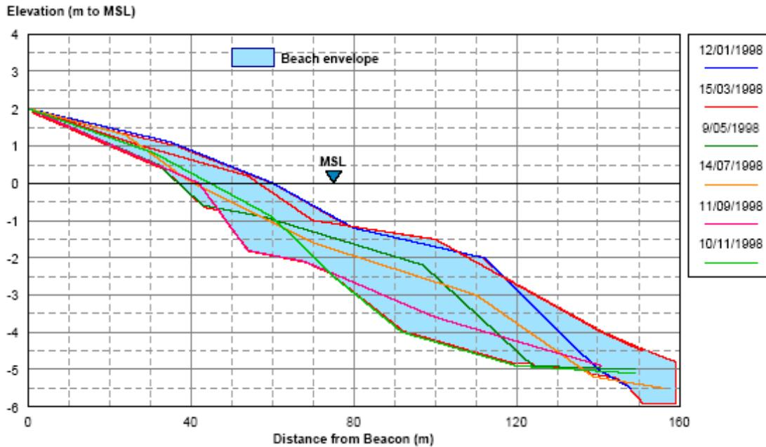
FIGURE 6.4: Example of beach profile envelope, showing maximum and minimum profiles
