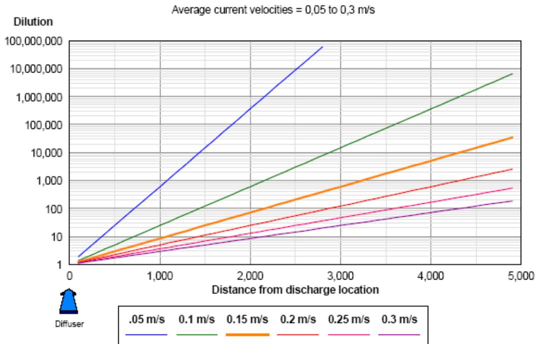
**FIGURE 6.50:** Dilutions due to decay versus distance under stronger current conditions.  $T_{90} = 2$  hrs (daytime).
