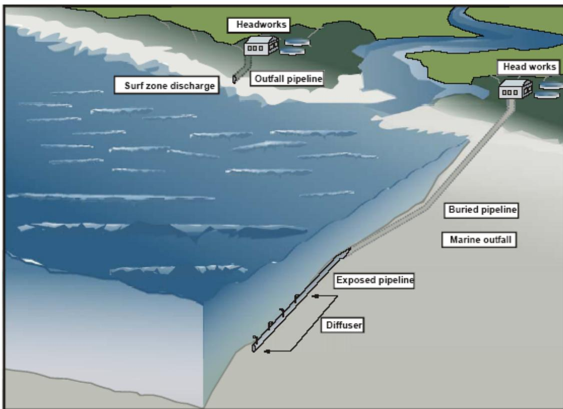
**FIGURE 6.30:** An illustration of the components of a well-designed wastewater discharge system
