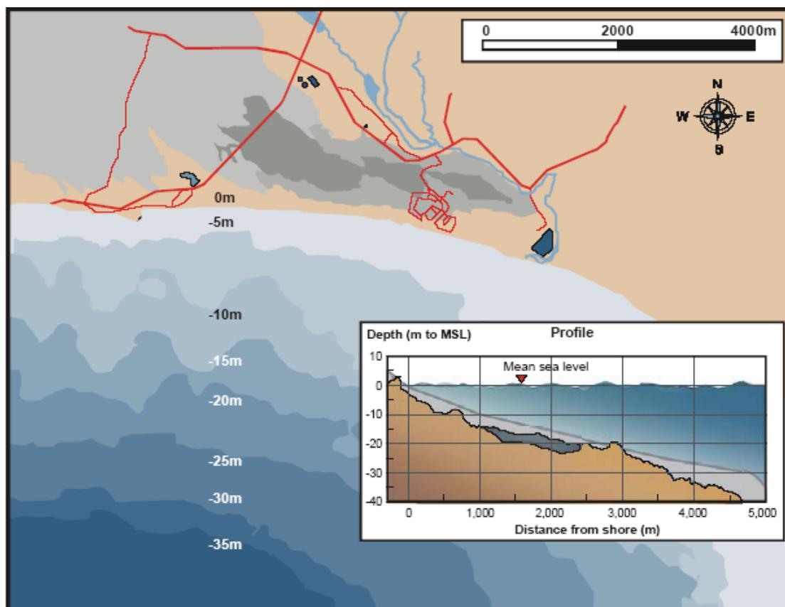
FIGURE 6.1: Example of bathymetric contour map and typical profile
