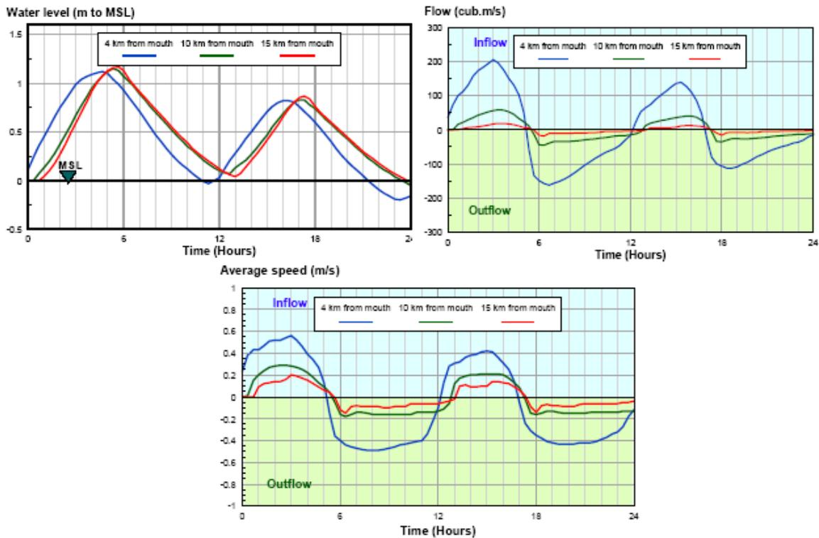
FIGURE 6.26: Water level simulations, flow rates and average stream velocities simulated at different locations in the Swartkops River Estuary under zero river inflow
