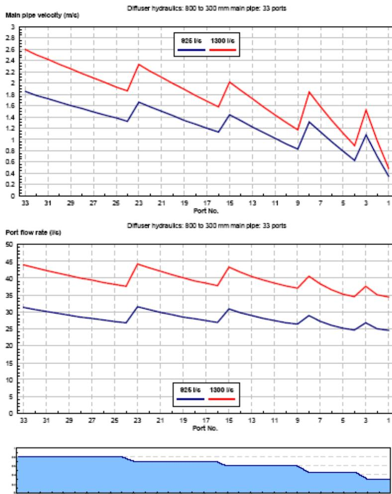
FIGURE 6.35 a: Example of graphical output required to evaluate hydraulic functionality: Main pipe velocities in the diffuser section (top) and port flow rates (bottom)
