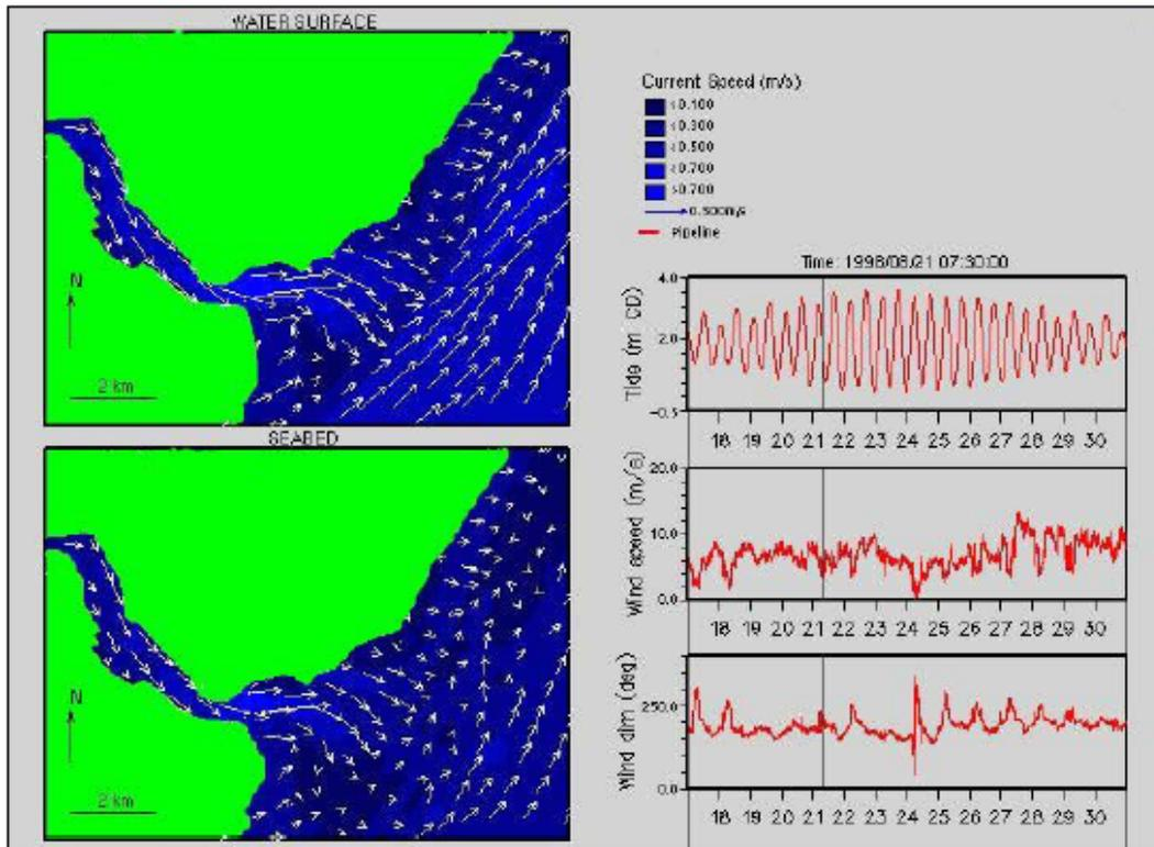
FIGURE 6.24 a: Example: Spatial output from a 3-D numerical model, showing current velocities and direction
