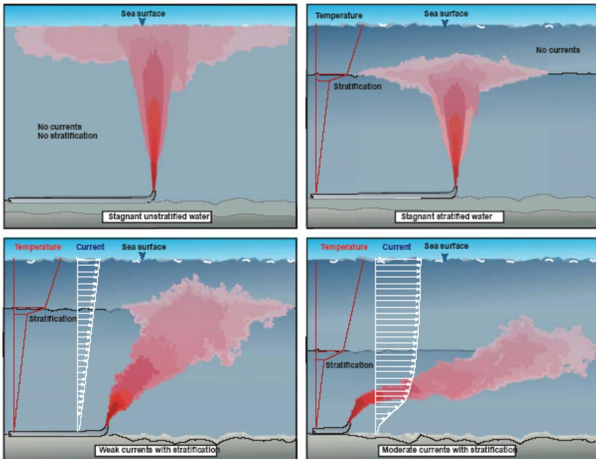
**FIGURE 6.38:** Buoyant plume in (a) stagnant, unstratified water, (b) stagnant, stratified water, (c) moving (weak currents) stratified water and (d) in moving (moderate currents), stratified water
