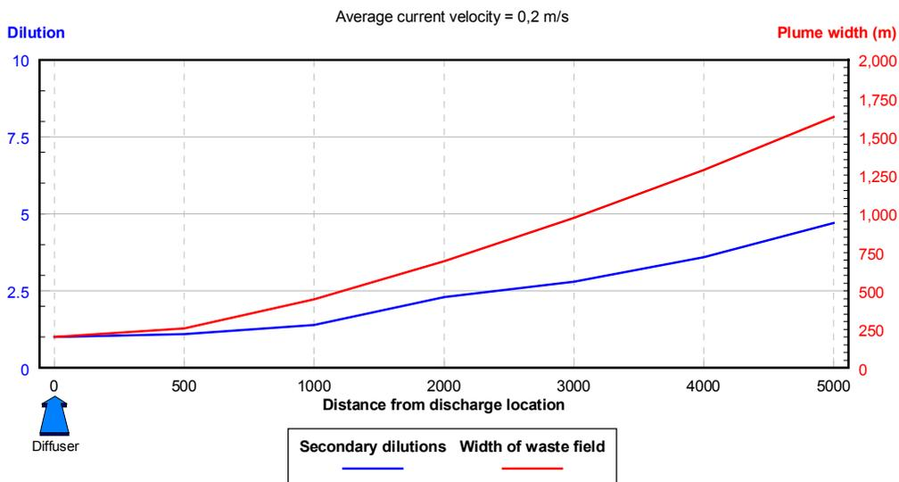
**FIGURE 6.41: Secondary dilutions and plume widths versus distance**
