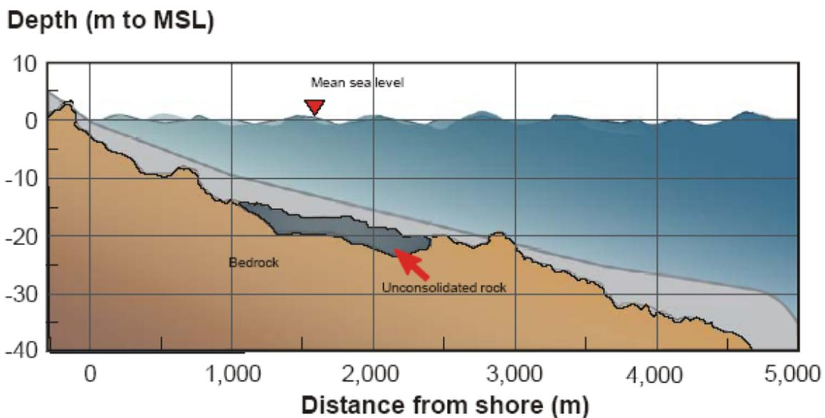
FIGURE 6.3: Sub-bottom profile derived from a seismic trace
