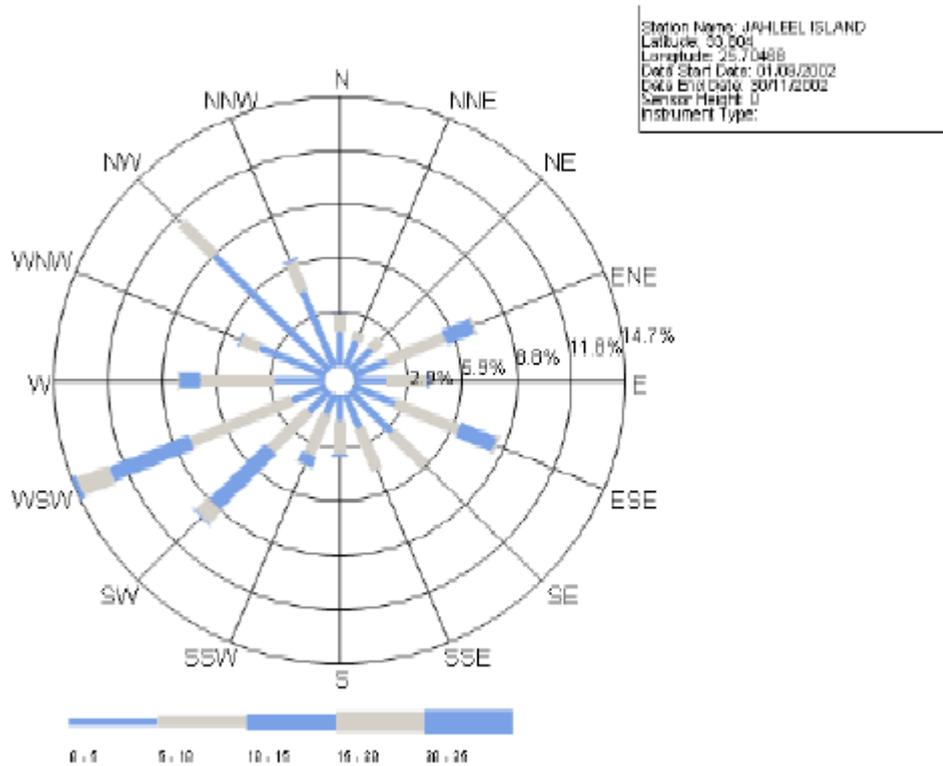
FIGURE 6.11: Wind-rose, showing the typical wind direction and speed at a particular site
