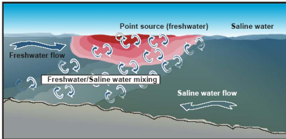
**FIGURE 6.47:** Illustration of the mixing of a wastewater plume in a partially stratified estuary
