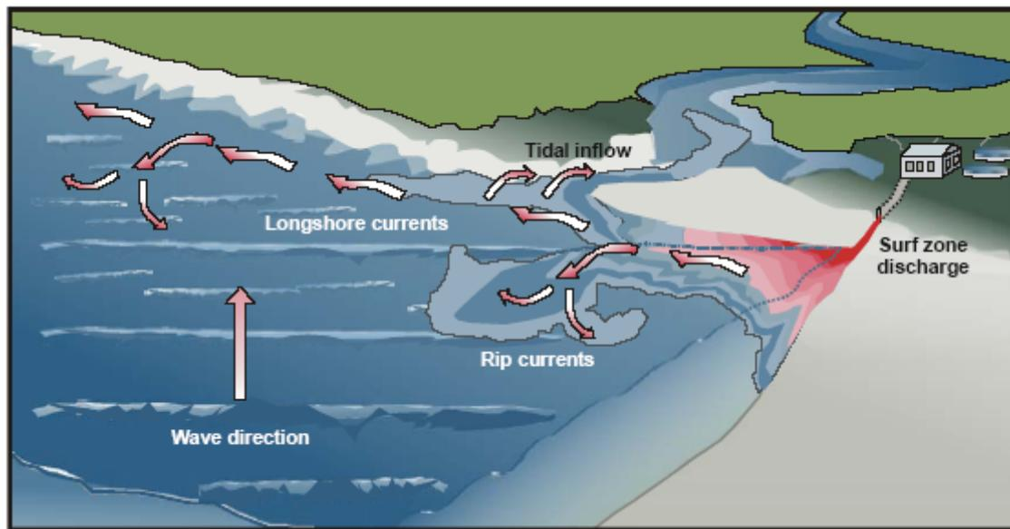
**FIGURE 6.37:** Illustration of the total dilution process for a surf zone discharge
