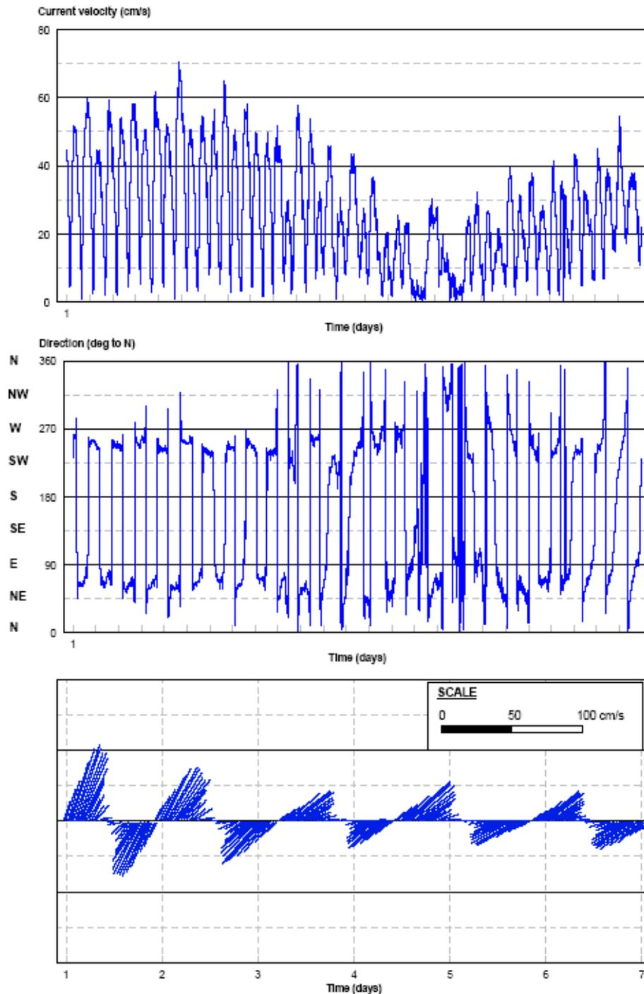
**FIGURE 6.15:** Time series data for current velocities, directions and vectors
