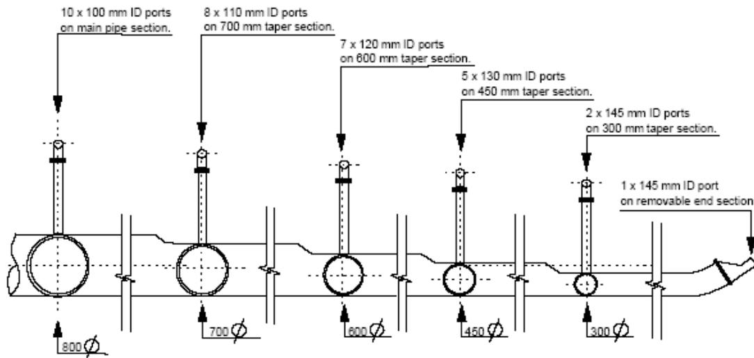
FIGURE 6.34: Typical diffuser layout
