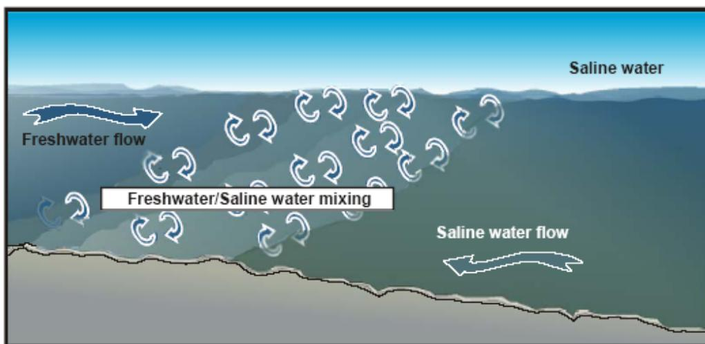
FIGURE 6.20: Illustration of vertical mixing in an estuary
