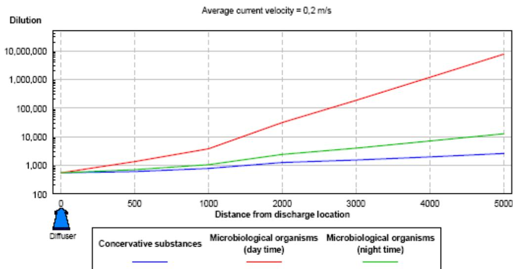
**FIGURE 6.52:** A graphical illustration of the achievable total dilutions versus distance
