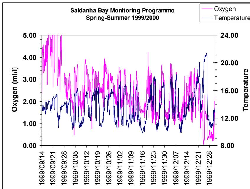
FIGURE 6.28: Dissolved oxygen variability in the bottom water layer in Saldanha Bay, South Africa (from Monteiro *et al.*, 1999)
