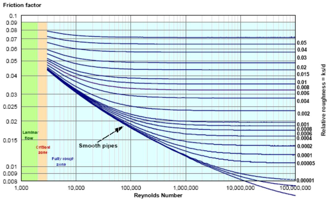
FIGURE 6.31: Moody diagram for pipe friction (Shand, 1993)
