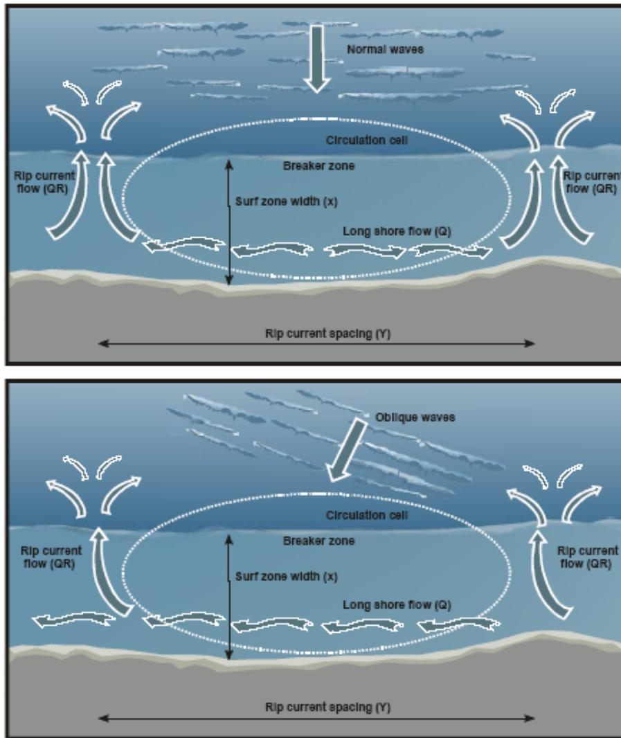
**FIGURE 6.45: Illustration of the longshore transport and dispersion processes in the surf zone under normal and oblique wave direction**
