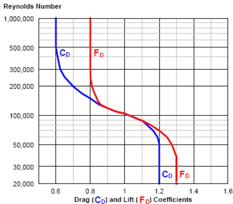
**FIGURE 6.59:** Drag and lift coefficients for an exposed pipeline on the seabed (Gunnerson, 1984)
