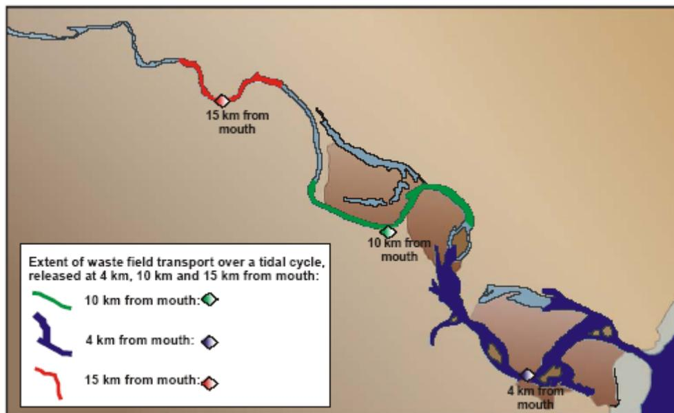
FIGURE 6.49: A simulation showing the difference in spatial behaviour of a wastewater plume released at different locations simulated in the Swartkops River Estuary
