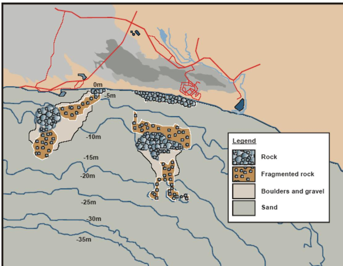
FIGURE 6.2: Example of a side scan sonar survey providing a graphic picture of the seabed characteristics
