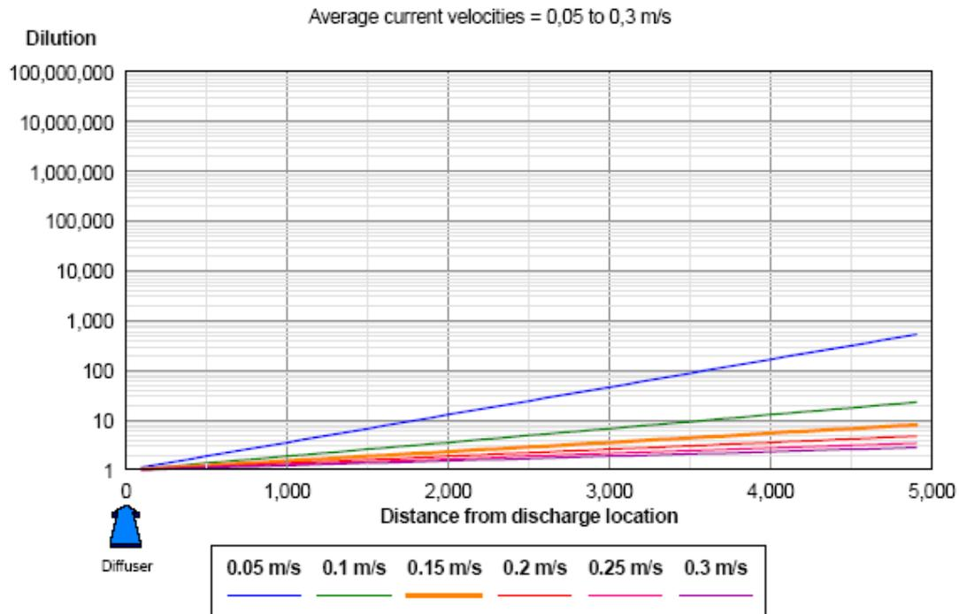
**FIGURE 6.51** Dilutions due to decay versus distance under weaker current conditions.  $T_{90} = 2$  hrs (daytime)
