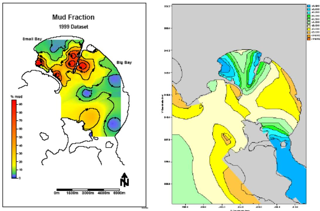
**FIGURE 6.29** Plots showing the measured particle size distribution in Saldanha Bay, as well as the modelled distribution of low turbulence (bed shear stress) zones in Saldanha Bay, South Africa (Monteiro *et al.*, 1999).
