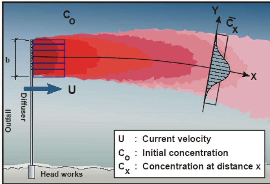
FIGURE 6.39: An illustration of Brooks's surface plume model
