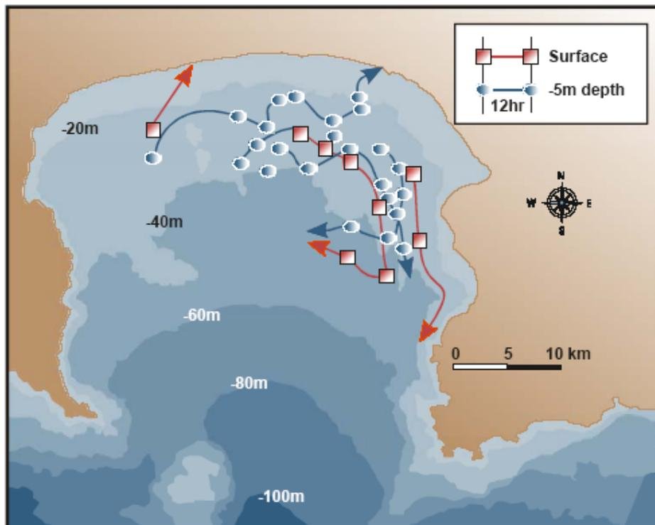
FIGURE 6.19: Circulation patterns recorded over three days in False Bay using radio-buoy tracking (Botes, 1988)
