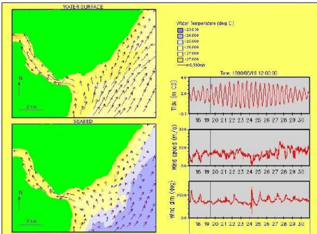
FIGURE 6.24 b: Example: Spatial output from a 3-D numerical model, showing temperature distribution
