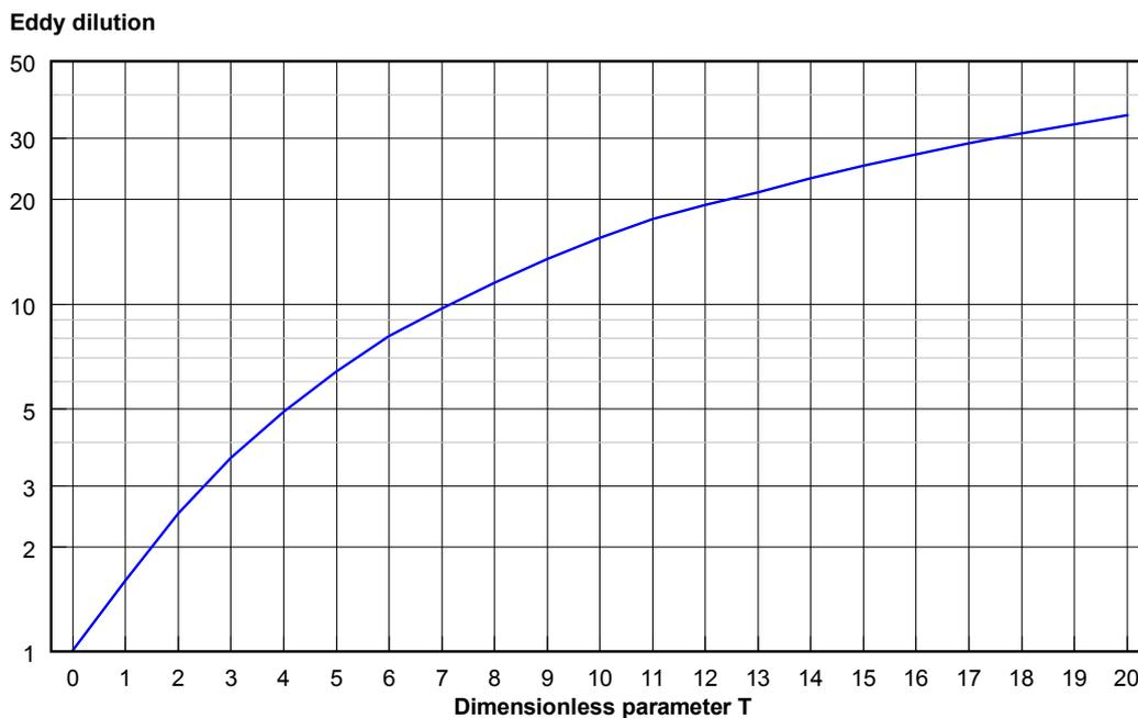
FIGURE 6.40: Graph from which to calculate secondary dilution using the dimensional parameter ( $T$ )
