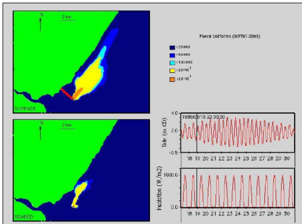
FIGURE 6.44: 3-dimensional simulation of an outfall plume
