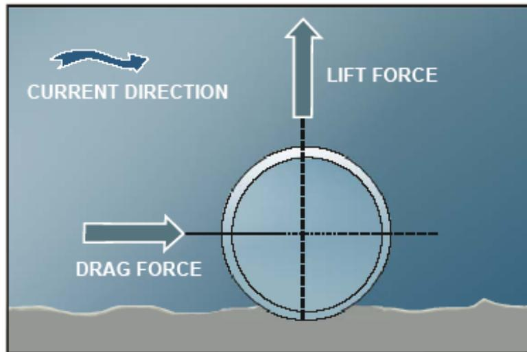
**FIGURE 6.58:** Drag and lift forces on a pipeline in steady flow
