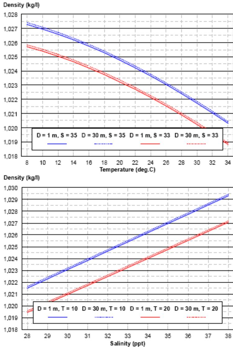
**FIGURE 6.21: Seawater density versus temperature and salinity**
