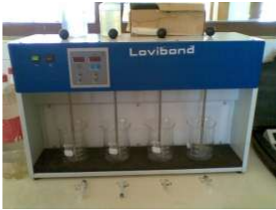
Jar testing is undertaken to ensure optimal flocculant dosing
