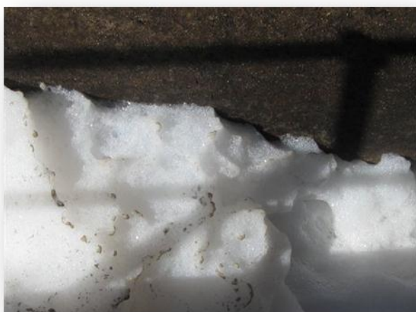
Absence of activated sludge and incorrect F:M ratios resulting in foam conditions
