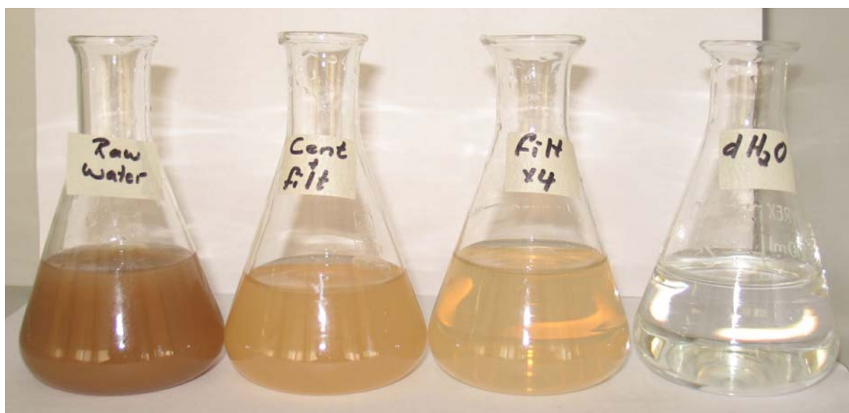
Figure 15: Water samples from the Caledon River: on the left is untreated water from the river (raw water) with a turbidity of 1 560 NTU. Second from the left is raw water centrifuged and then filter trough a GF/C glass fibre filter. Third from the left is raw water centrifuged and filter 4 times through GF/C filters. Note the high turbidity still present in the water, indicating coloured organic material and very fine suspended material. On the right is distilled water for comparison.
