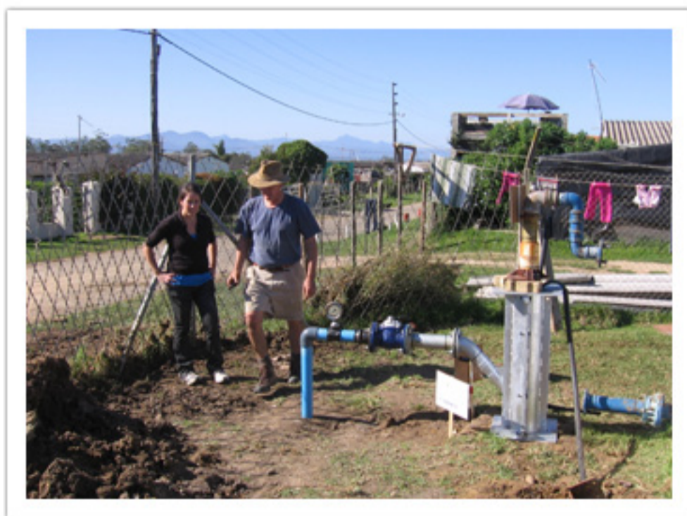
Photo 9: Borehole injection test in Plettenberg Bay
