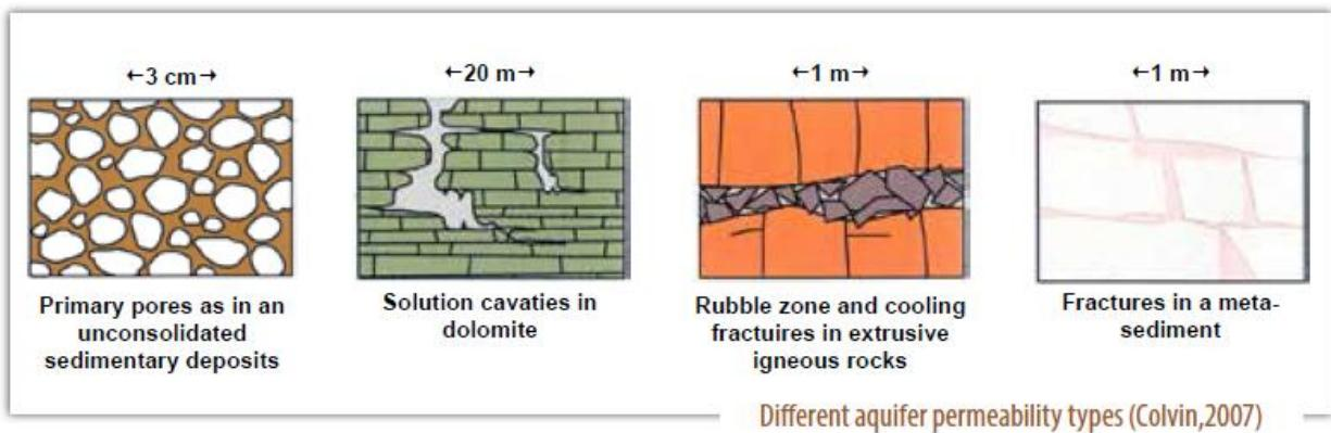
**Figure 2: Different aquifer permeability types (Colvin, 2000)**
