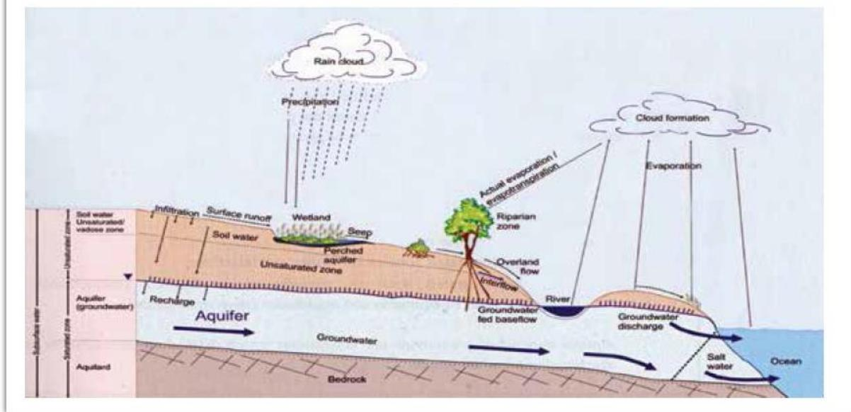
**Figure 5: Subsurface and surface flows of water in the environment (Colvin, et al., 2007)**
