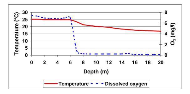
Figure 2. The temperature and dissolved oxygen concentration at Site 2 in the Lindleyspoort Dam at the dam wall on 14/02/2001.
