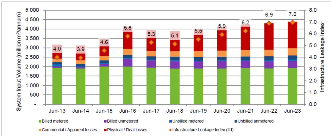
**Figure 7.11: The Infrastructure Leakage Index**
