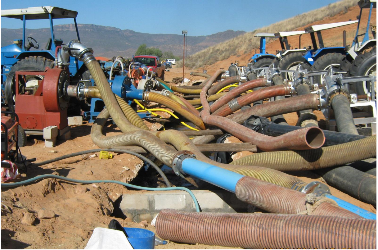
Figure 7-3: “Pump garden” to pump water across broken canal section
