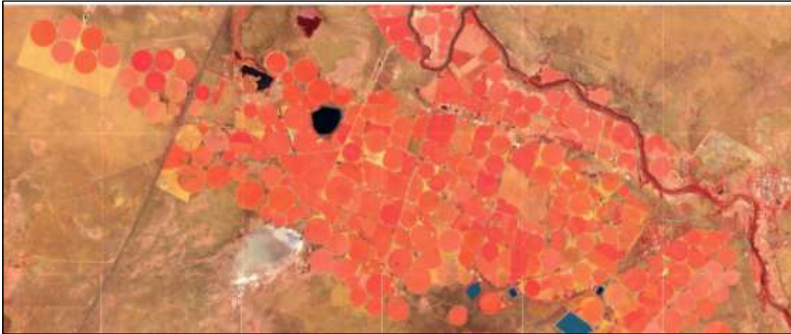
Figure 11: Irrigation scheme along the Riet River illustrated with a false colour Sentinel-2 satellite image composite (bands 8, 4 and 3) where red indicates healthy vegetation.
