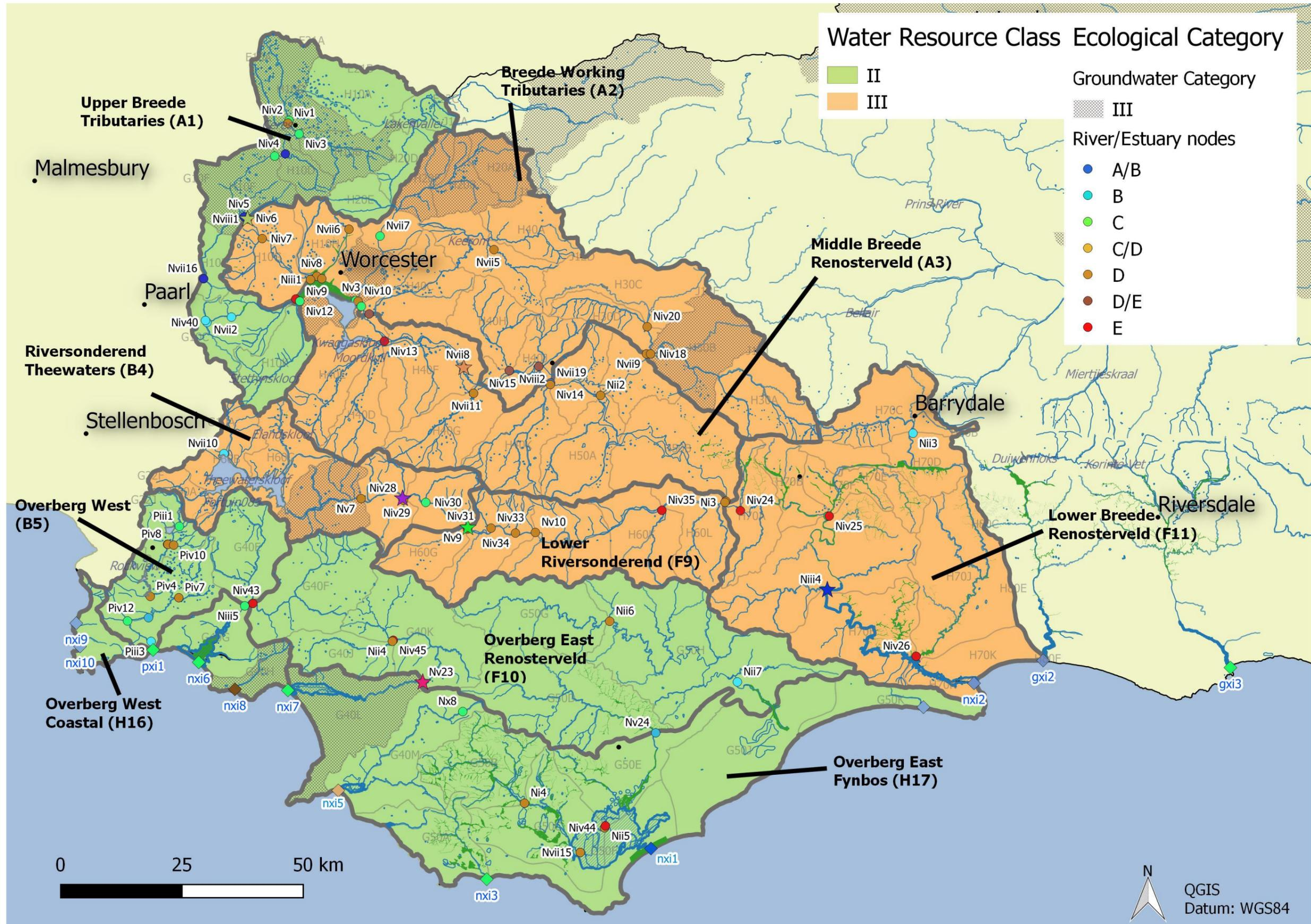
Figure 1.2 Locations of IUAs (with their recommended Class) and biophysical/ allocation nodes in the Breede River catchment and Overberg area
