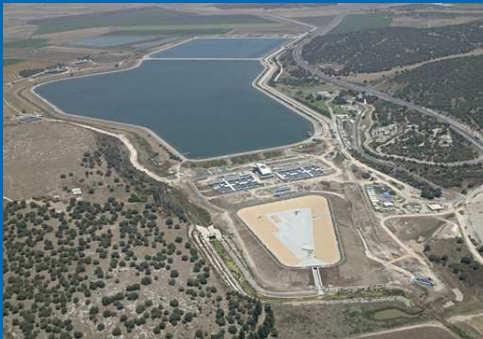
Palmachim SWRO plant is modular and easily expanded from 30 to 60 Mm 3 /Year
