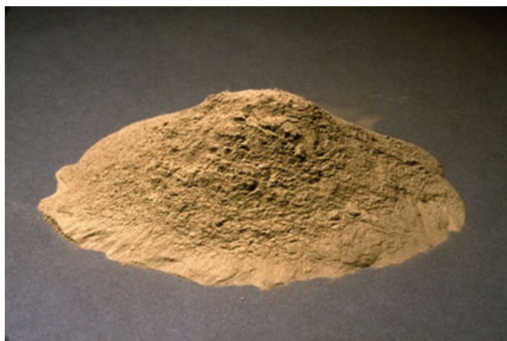
Figure 7: Fly ash recovered during sludge combustion
