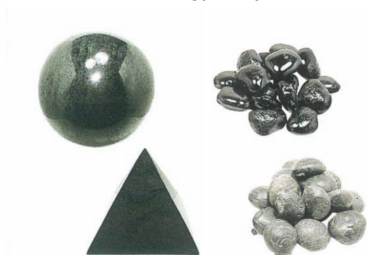
Figure 16: Marble-like material manufactured from sludge
