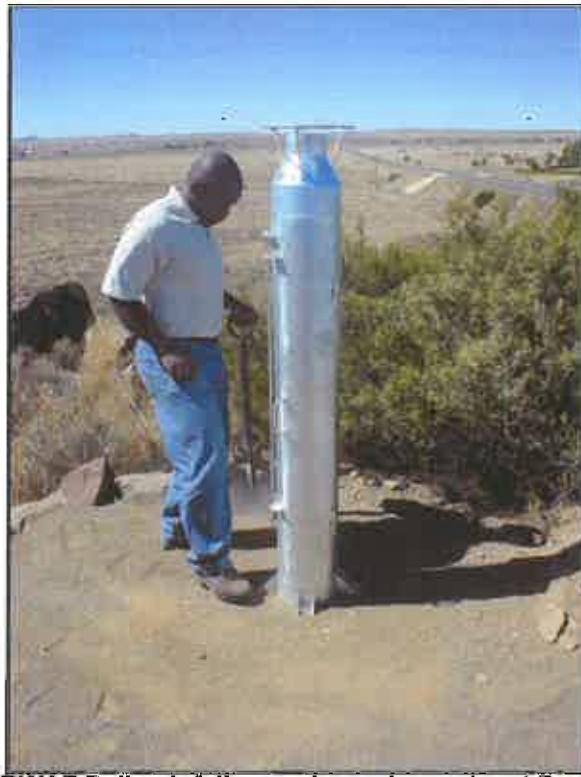
Plate 2: DWAF Bulk rainfall recorder and sampler at De Aar (photo F. Fourie, DWAF)
