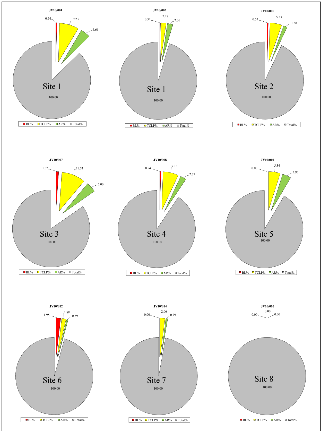
Figure 4. Pie charts of extractable (mobile) fractions of total nickel concentration per sediment sample as produced by the three leach test methods used. Note that each 'sliver' is a fraction of 100%.
