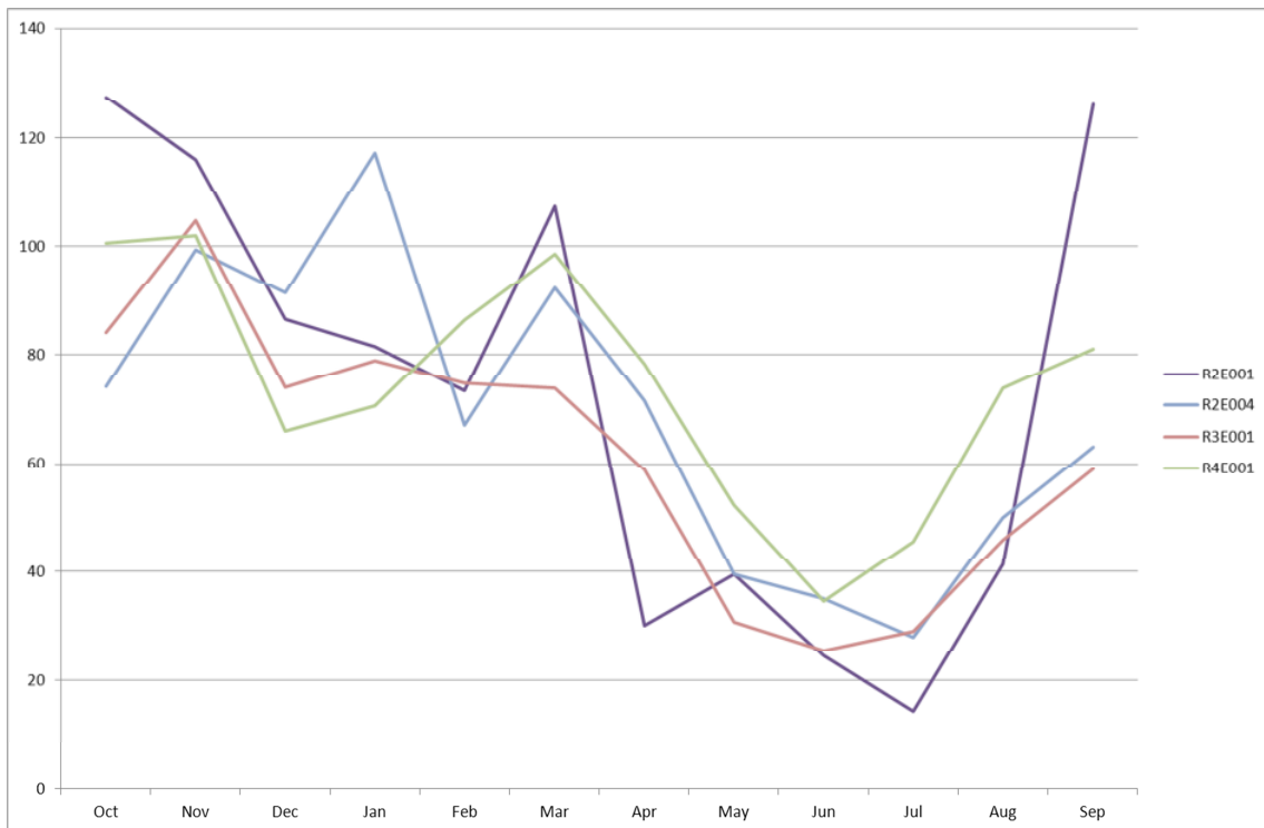
Figure 4-6 Average seasonal rainfall pattern (mm/a) in Drainage Region R; a) inland climate stations, b) coastal stations (around East London)
