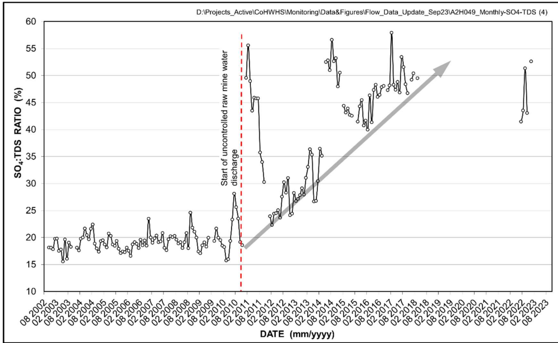
Figure 19 Pattern and trend of the SO 4 : TDS ratio at station A2H049 since the start of mine water decant in the Western Basin in mid-2002
