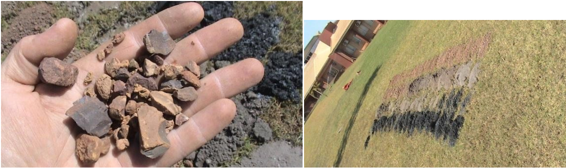
Plate 1: Washed colluvium, fine-grained matrix removed, predominantly consisting of fragments of lava and quartzite, the underlying grey to brown (weathered) and black formation (fresh) in the samples on the right is shale. Photo taken at Thabazimbi hospital, May 2013.
