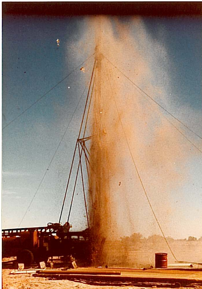
PLATE 10: Detonation at approximately 30 m in G34354, Site 4
