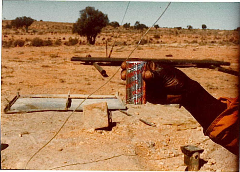
PLATE 5: Individual charge of Pentolite explosive
