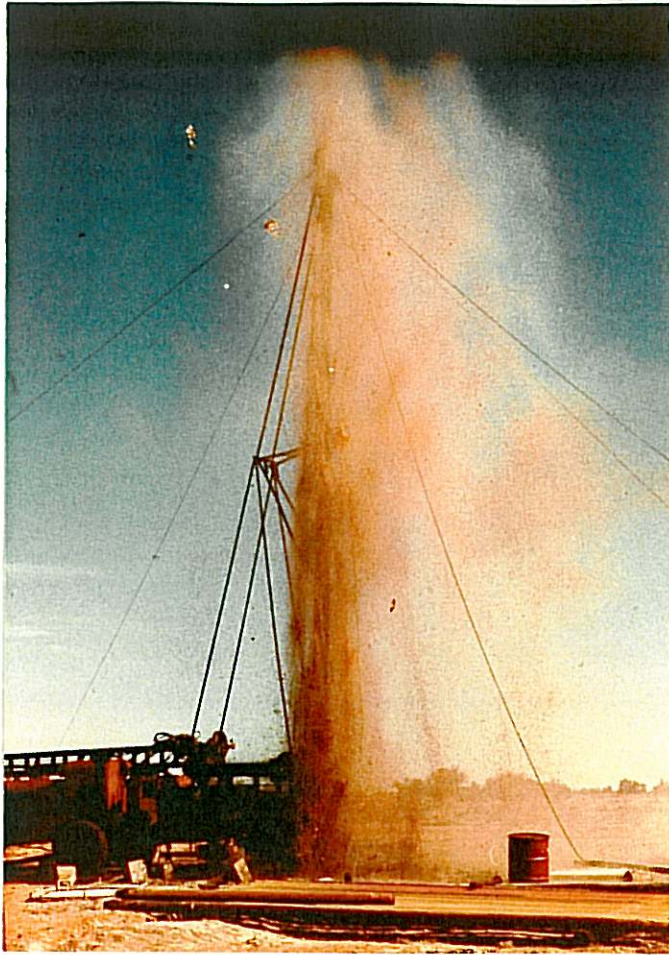
PLATE 10: Detonation at approximately 30 m in G34354, Site 4
