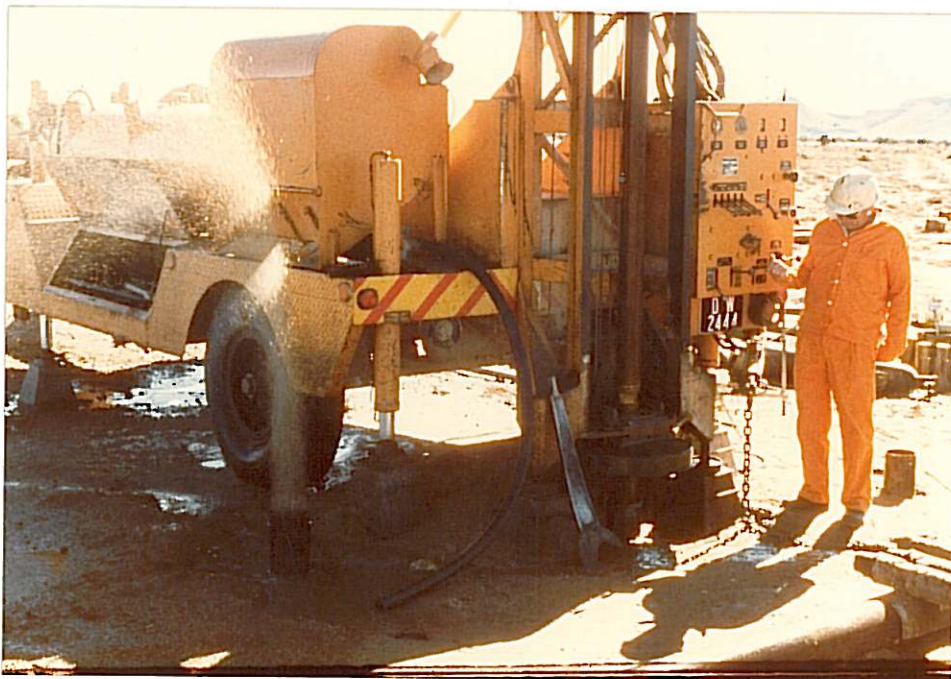
PLATE 13: Water ejected from G34350 (Left) while 'blowing' G34348. Boreholes are 1,75 m apart
