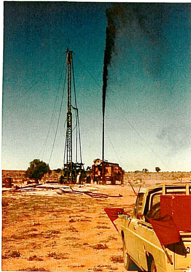
PLATE 9: Detonation at a depth of 124 m in G34357, Site 4
