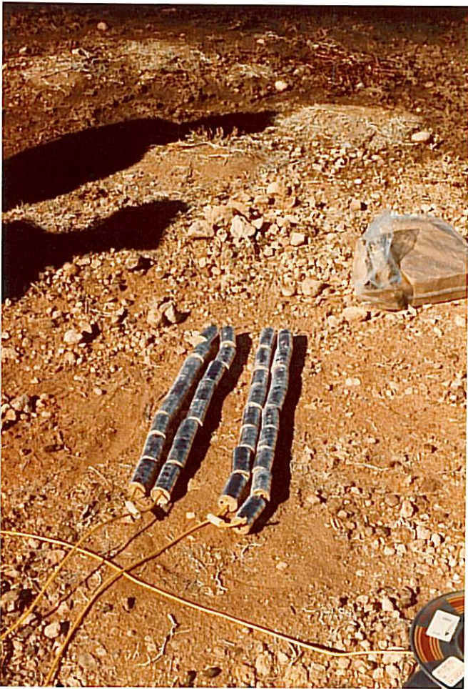
PLATE 6: Approximately 5 kg of Pentolite explosive, with cortex connection, ready for packing
