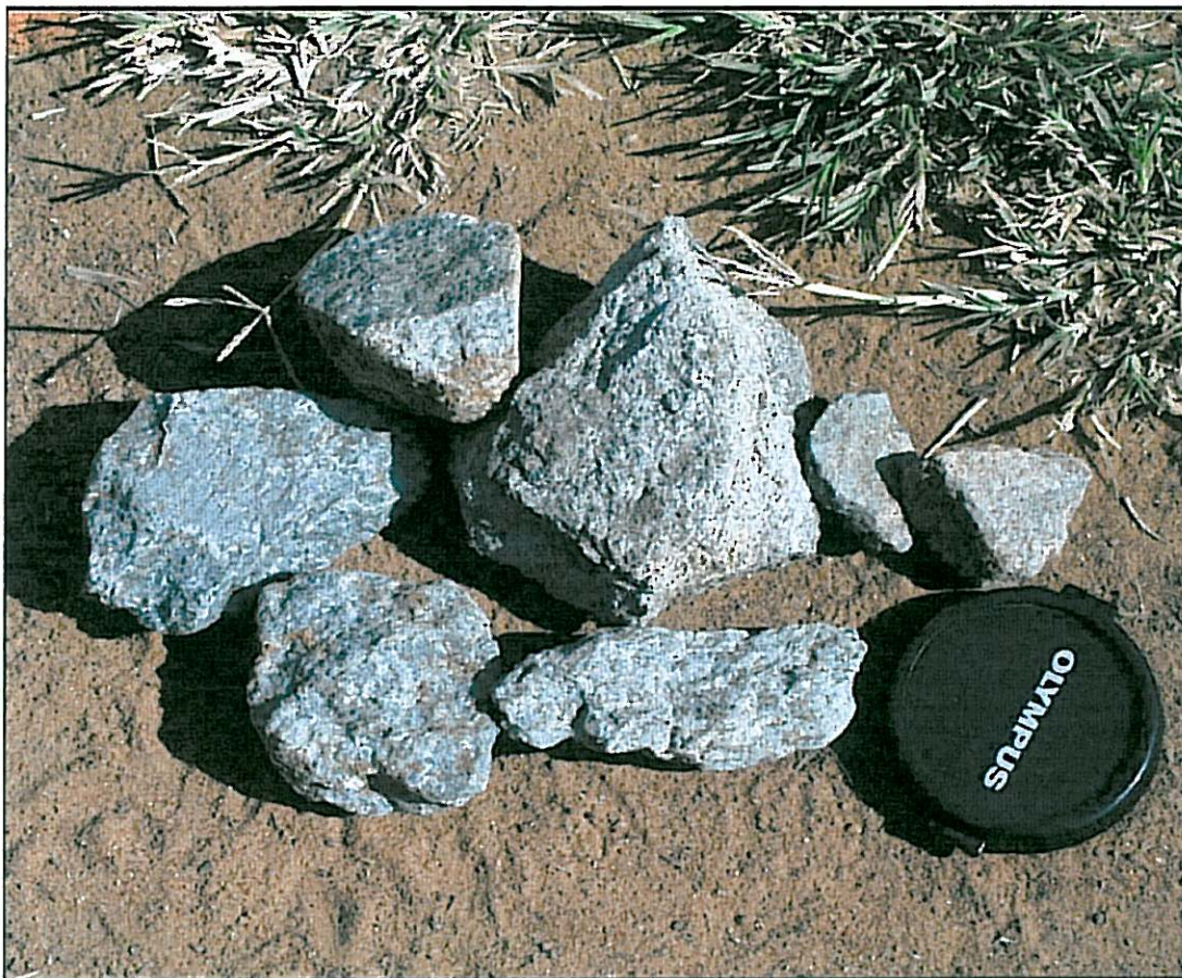
Plate 3.1 Basement granite-gneiss samples from a borehole on the farm Middel Kop.
