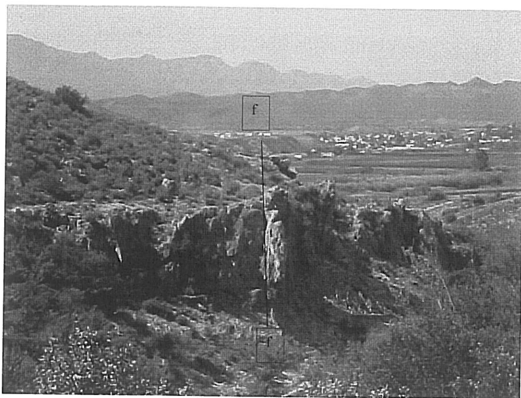
Figure D12 View of fault plane in TMS near borehole KG 1, Calitzdorp. Fault strikes 51^{\circ} , dip \approx 80^{\circ} . Borehole KG1 is situated to the right of this fault plane.
