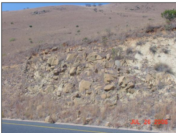
Photo 12: Proterozoic dyke in the Kaap Valley Granite between Badplaas and Barberton. Dykes are important targets for successful groundwater development in the map area (photo W.H. Du Toit, 2006).
