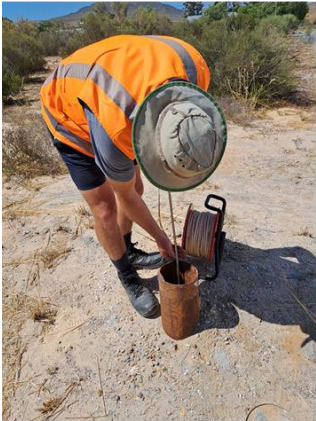
(a) Measuring water level
