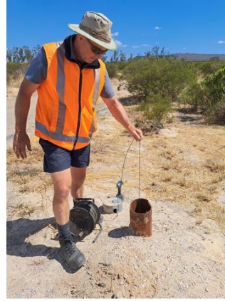
(a) Measuring borehole depth
