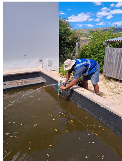
(b) Well point outflow sampling point
