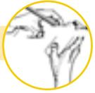
tap with a solution of sodium hypochlorite (100 mg/1 NaOCl) before sampling (Ask laboratory for more detail). Let the water run for 2 to 3 minutes afterwards.
