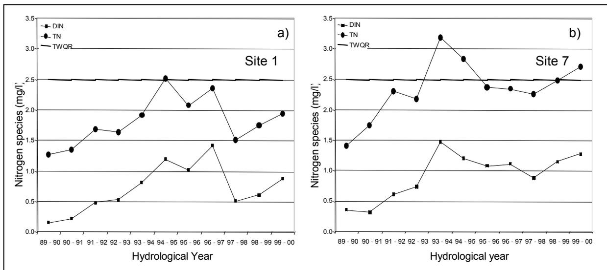
Figure 5. Mean annual concentration for TN (KN & NO<sub>3</sub>-N+NO<sub>2</sub>-N) and DIN (NO<sub>3</sub>-N+NO<sub>2</sub>-N & NH<sub>4</sub>-N) in the Roodeplaat Dam (1989 – 1999) compared to the TWQR for dissolved inorganic nitrogen (DWAF 1996c) at a) Site 1 and b) Site 7.
