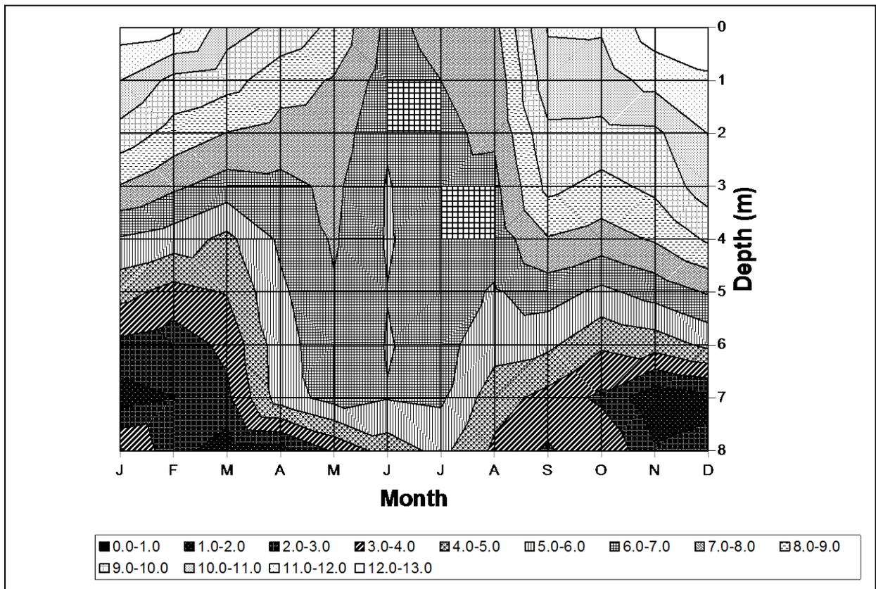
Figure 14. Mean monthly oxygen profiles in the Roodeplaar Dam at Site 7 (1990 to 1998). The oxygen concentration is expressed as mg/l of dissolved oxygen.
