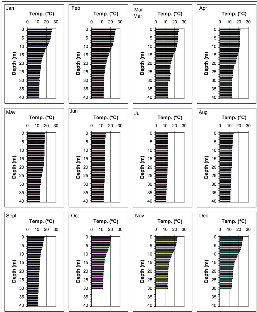
Figure 11. Mean monthly temperature profiles in the Roodeplaats Dam at Site 1 (1980 to 1997)
