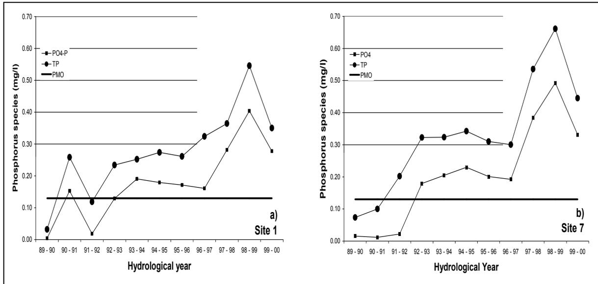
Figure 2. Changes in mean annual TP and PO4-P concentrations in the Roodeplaat Dam (1989–1999). a) Site 1 b) Site 7. PMO = Phosphorus Management Objective for TP concentrations.
