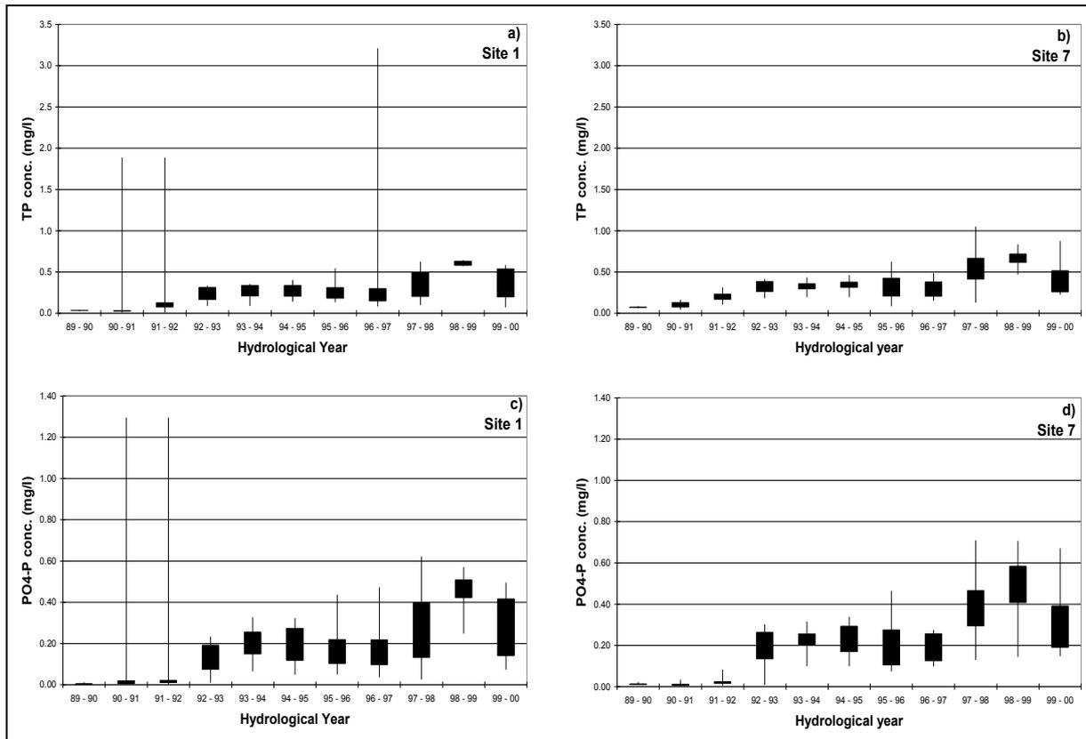
Figure 3. Boxplots showing the historical trends of the TP and PO4-P concentrations in the Roodeplaat Dam at Site 1 (a and c) and Site 7 (b and d). The boxplots show the minimum, maximum, 25th percentile and the 75th percentile for each hydrological year.
