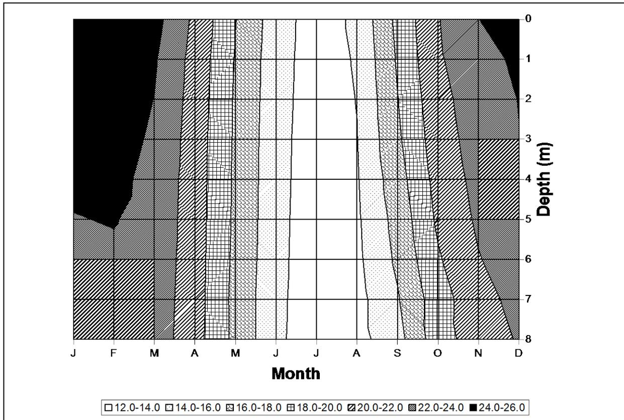
Figure 13. Mean monthly temperature profiles in the Roodeplaas Dam at Site 7 (1990 to 1998). The temperature is expressed in degrees Centigrade.
