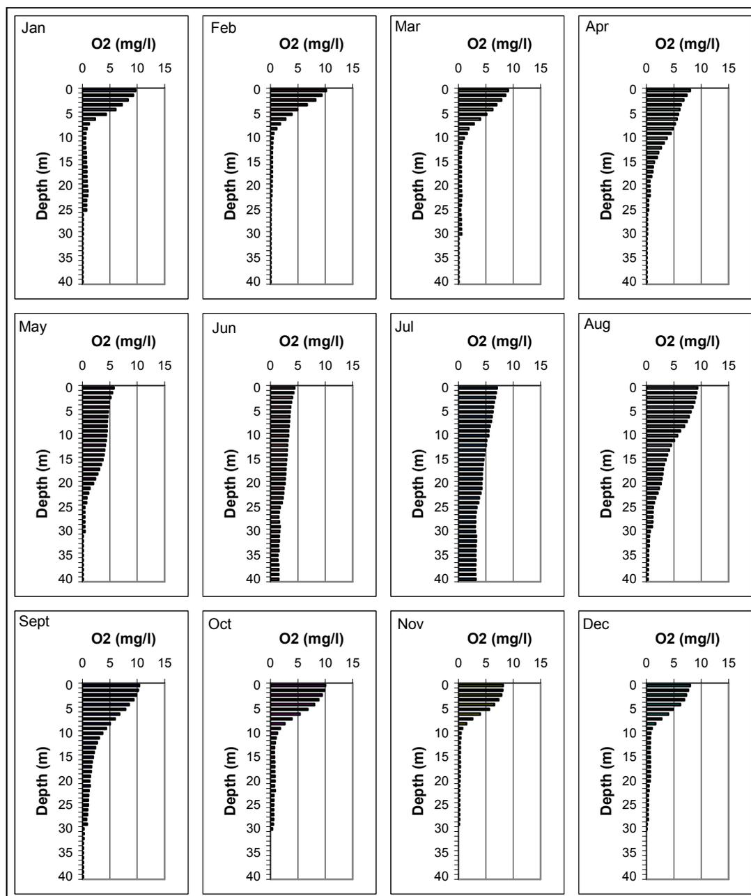
Figure 12. Mean monthly oxygen profiles in the Roodeplaats Dam at Site 1 (1980 to 1997).
