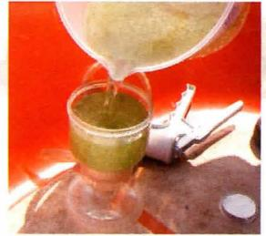
Use the vacuum pump to draw water through the filter. Filter 500 ml if possible. **The total amount filtered must be recorded on the tag.**
