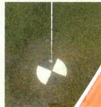
Record the depth by counting the markings on the wet part of the rope (markings at 10cm intervals)
