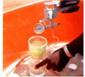
Open filter unit. Gently lift one side of the filter paper and remove the filter paper from
