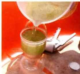
Use the vacuum pump to draw water through the filter. Filter 500 ml if possible. **The total amount filtered must be recorded on the tag.**
