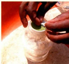
Push the rolled filter into the glass tube and shake gently until the filter paper is immersed in the ethanol.
