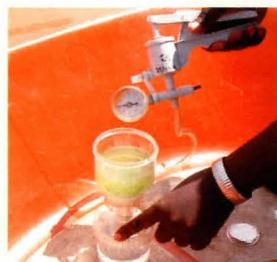
Open the filter unit. Gently lift one side of the filter paper
