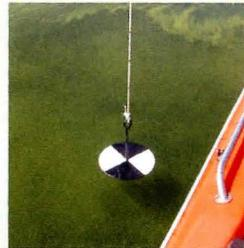
The secchi is lowered into the water until the black and white quadrants are just visible
