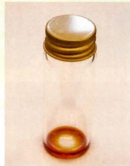
It is possible for the lugol solution to leak out or dry out. In such instances the monitor can add lugol using a dropper
