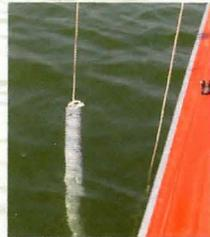
Hold the top end steady while pulling the weighted end up till both ends are at the water surface
