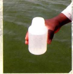
Preserve with one ampoule of mercury chloride. Drop the entire ampoule into the bottle after broken (see page 21)
