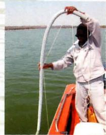
Lower the pipe until the top end is level with the water surface
