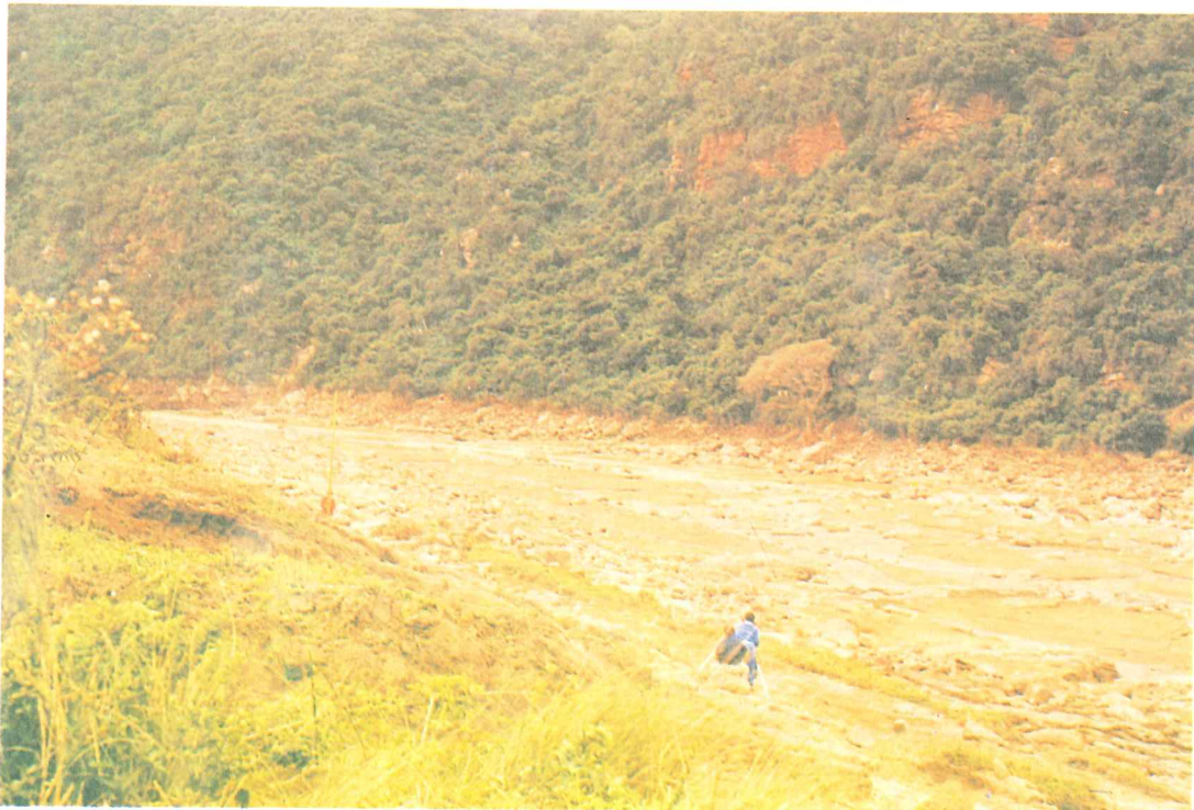
44. Mgeni River: Site 40, slope-area site downstream of Inanda Dam, looking upstream from right bank. Representative roughness = 0,7 m
