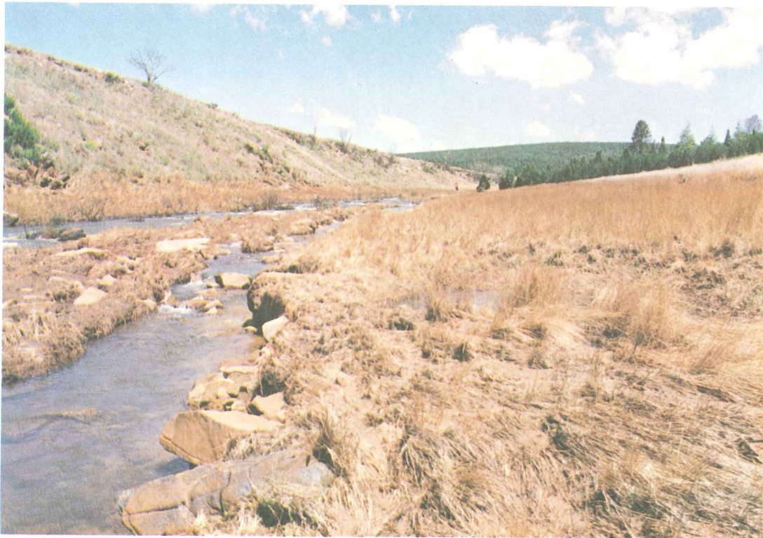
52. Mvoti River: Site 43b, which is an excellent slope-area site viewed from right bank looking upstream. Representative roughness = 0,3 m
