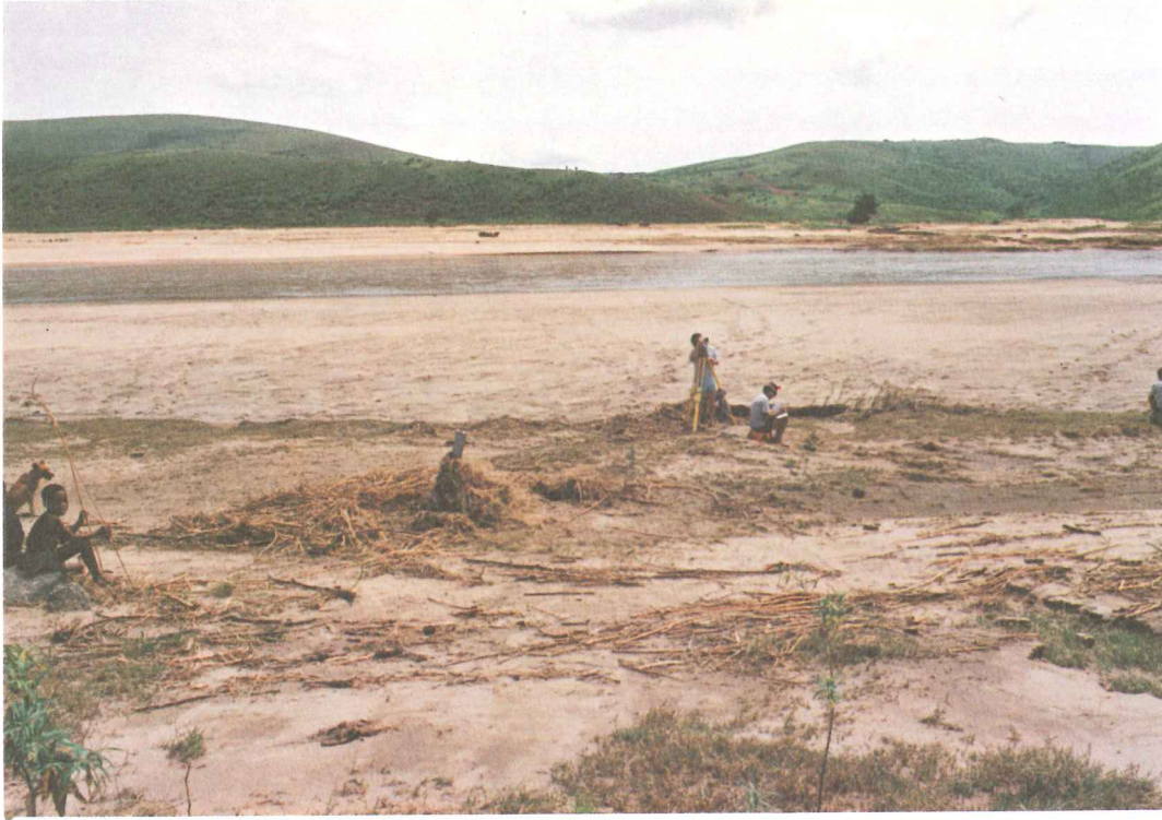
73. Mfolozi River: Site 91. Significant deposition of sediment occurred on the floodplains and river banks. Representative roughness = 0,4 m
