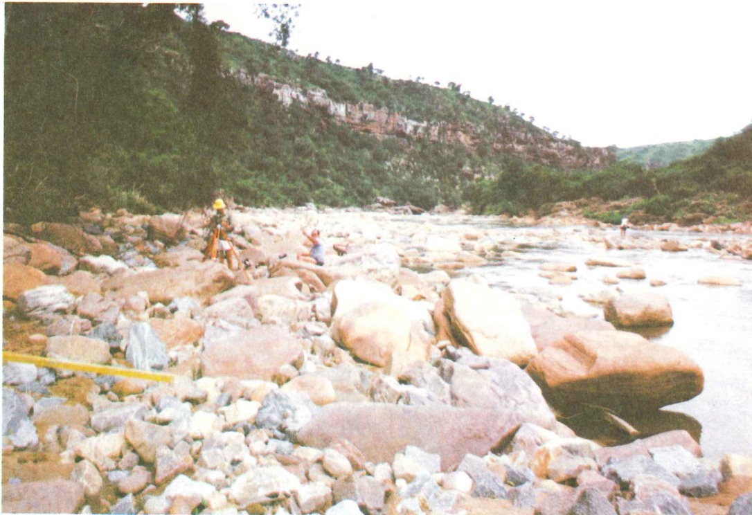
28. Mlazi River: Site 22b, slope-area site, 300m down stream of Nshongweni Dam. Representative roughness = 1.5 m
