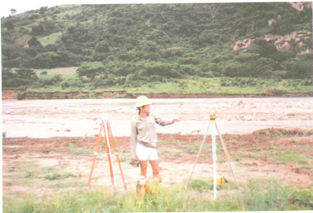
42. Mqeku River: Site 38, cross section 3 viewed from right bank. This is a excellent slope-area site. Representative roughness = 0,5 m
