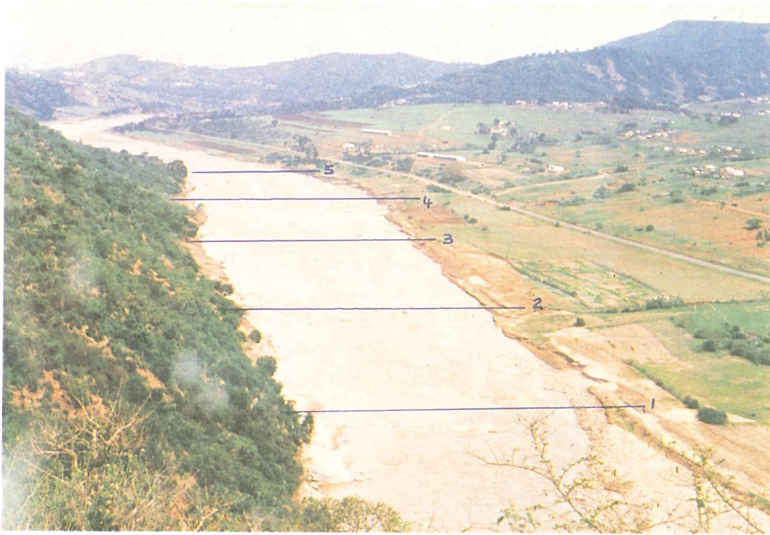
35. Mgeni River: Site 33, downstream of Nagle Dam showing sections of an excellent slope-area site. Representative roughness = 0,9 m
