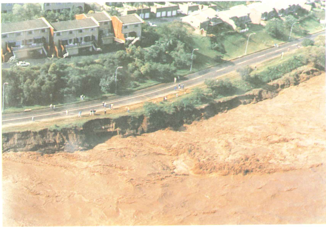
45. Mgeni River in Durban North showing bank erosion at Riverside road (Photograph by South African Transport Services - SATS)
