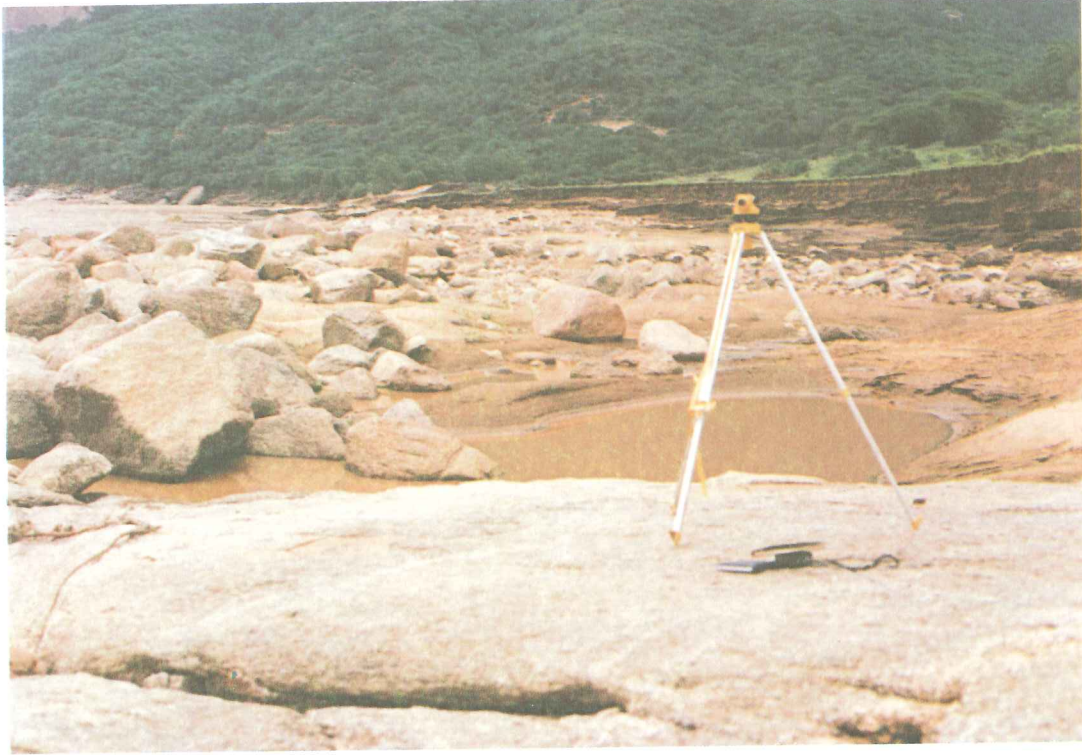
41. Mgeni River: Site 37, downstream of confluence with Msunduze River, viewed from right bank, looking downstream. Representative roughness = 0,9 m
