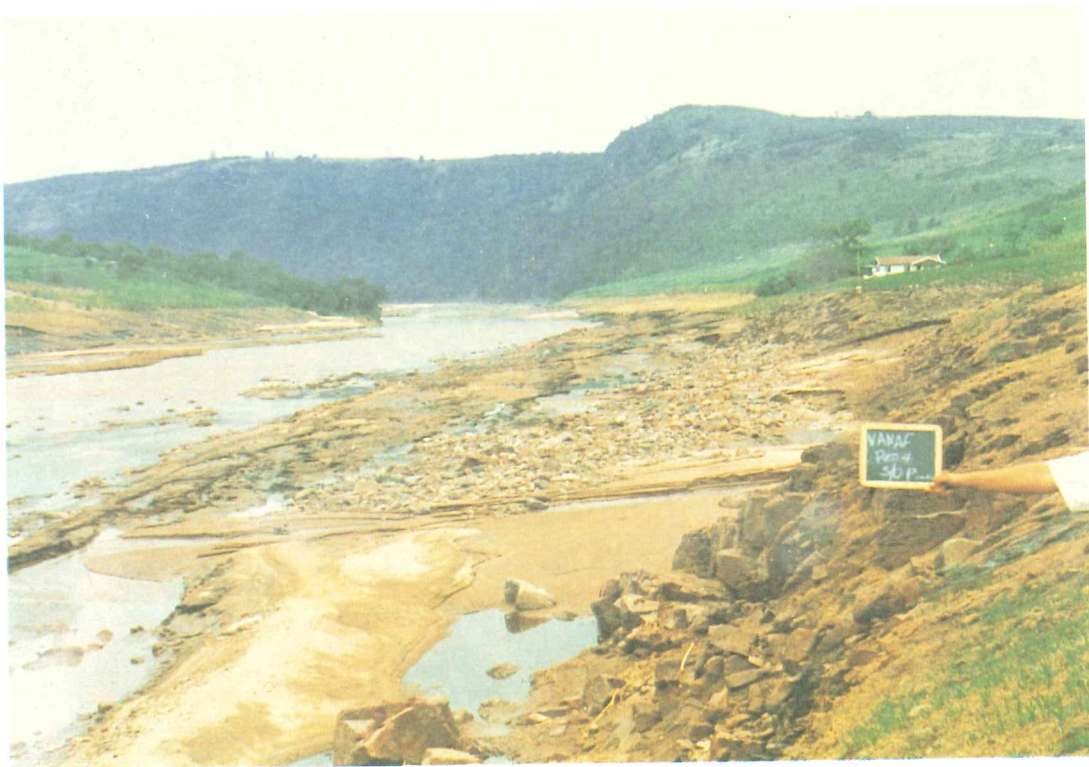
54. Mvoti River: Site 44, slope-area site at Wellvale near Stanger, viewed from left bank looking upstream. Representative roughness = 0,5 m
