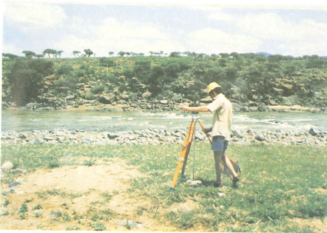
59. Mooi River: Site 68, at Keates Drift, view of cross section 3 from left bank, of an excellent slope-area site. Representative roughness = 0,7 m
