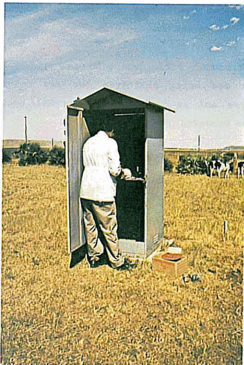
PLATE 2: Changing the chart of a groundwater recorder
