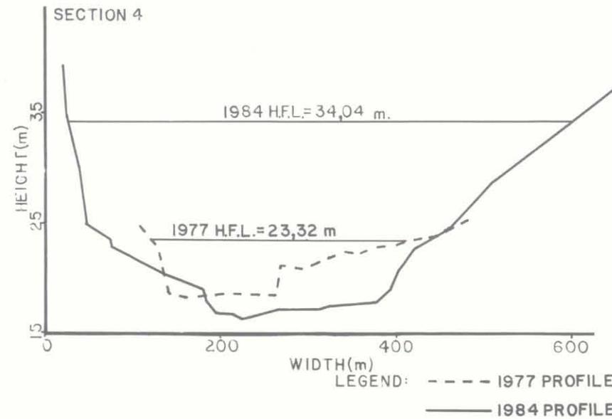
FIG.7.5 c COMPARISON OF CROSS SECTION CHANGES AT SITE 18: MFOLOZI RIVER
