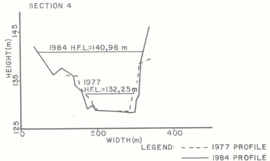
FIG.7.5 a COMPARISON OF CROSS SECTION CHANGES AT SITE 13: WHITE MFOLOZI RIVER
