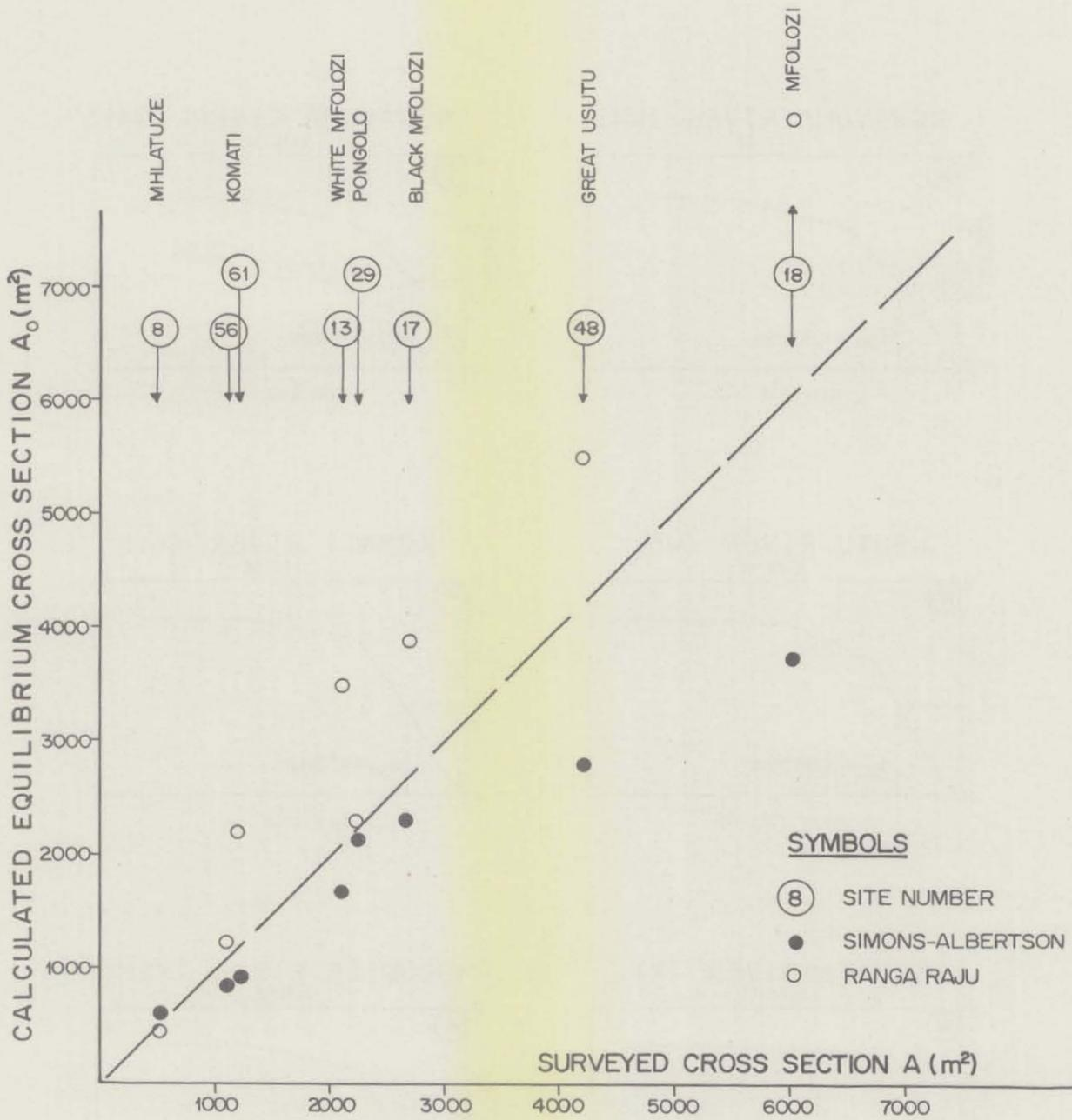
FIG. 7.3 SURVEYED vs CALCULATED CROSS SECTIONAL AREAS IN ALLUVIAL RIVERS
