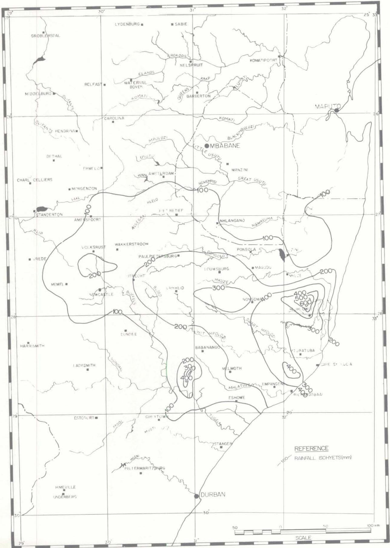
FIG. 2.5 ISOHYETAL MAP OF THE 2-5 JULY 1963 STORM
