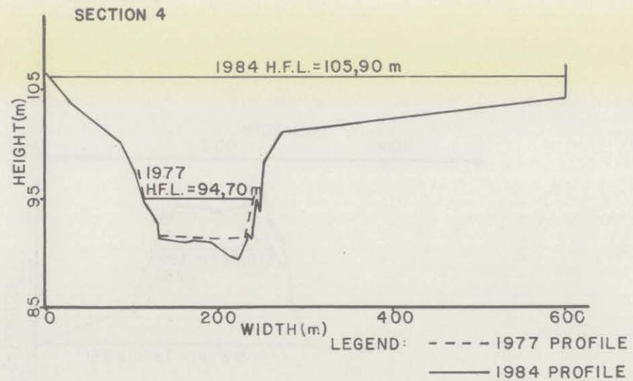
FIG.7.5 b COMPARISON OF CROSS SECTION CHANGES AT SITE 17: BLACK MFOLOZI RIVER
