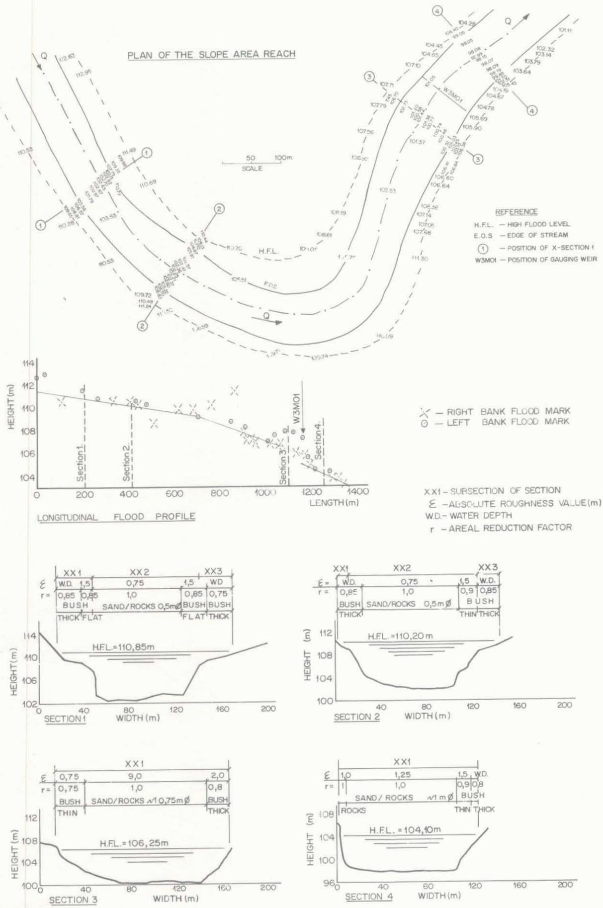
FIG. 4.3 SLOPE AREA SURVEY AT SITE 22 : PLAN AND SECTIONS
