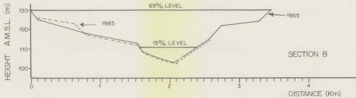
FIG. 7.4 c2 PONGOLAPOORT DAM: CROSS SECTIONS 2,3, A AND B
