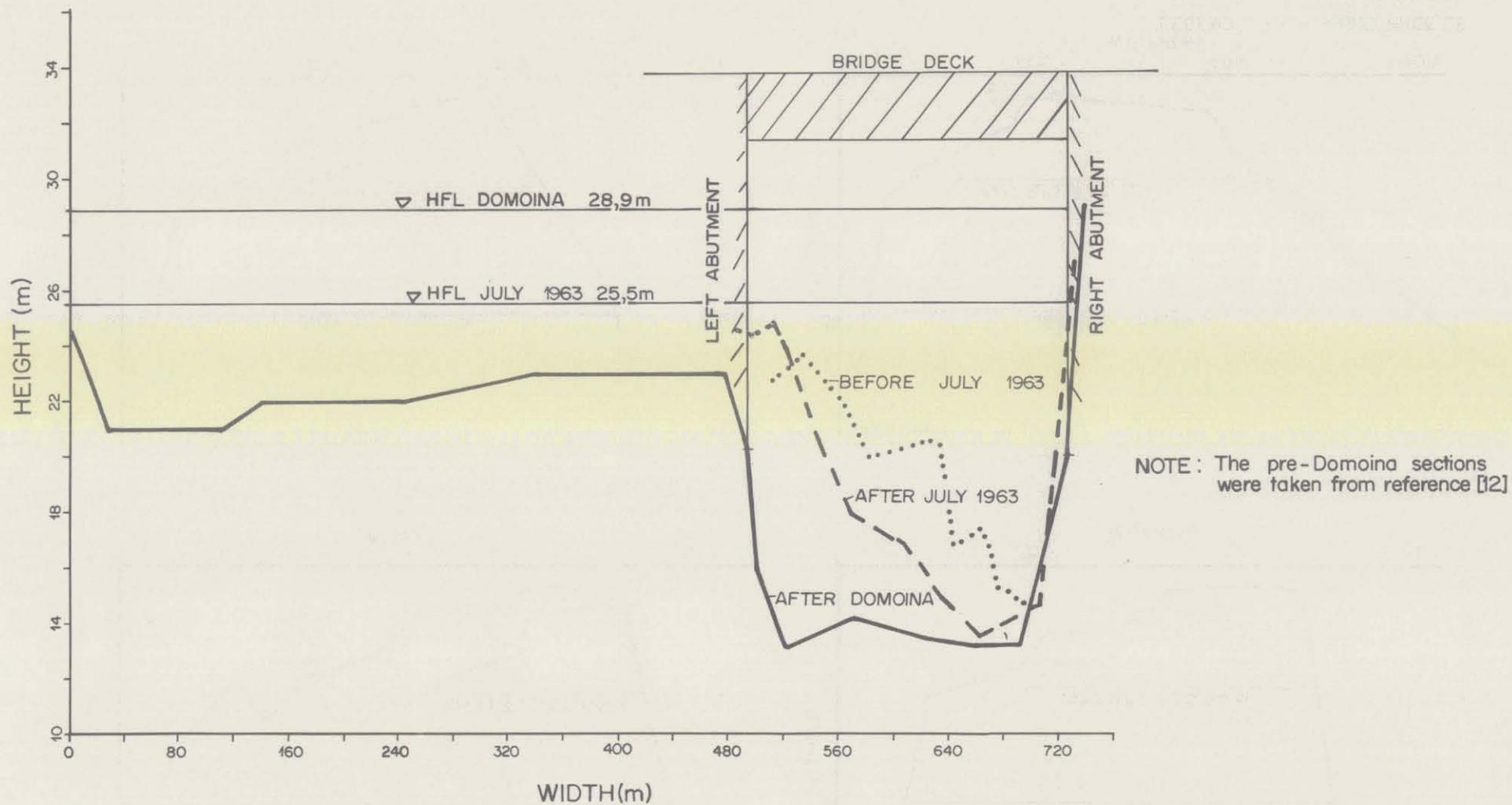
FIG. 7.6 COMPARISON OF SURVEYED SECTIONS AT SITE 19 (MFOLOZI AT THE N2 BRIDGE)
