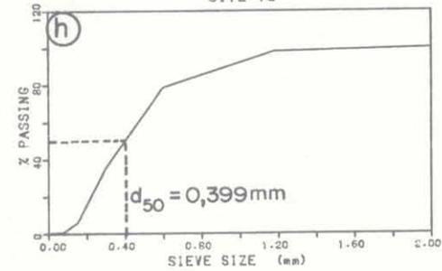
FIG. 7.2 (a-h) SEDIMENT GRADING CURVES
