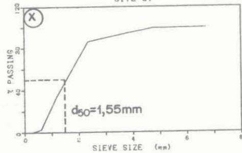
FIG. 7.2 (q-x) SEDIMENT GRADING CURVES
