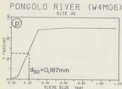
FIG. 7.2(i-p) SEDIMENT GRADING CURVES
