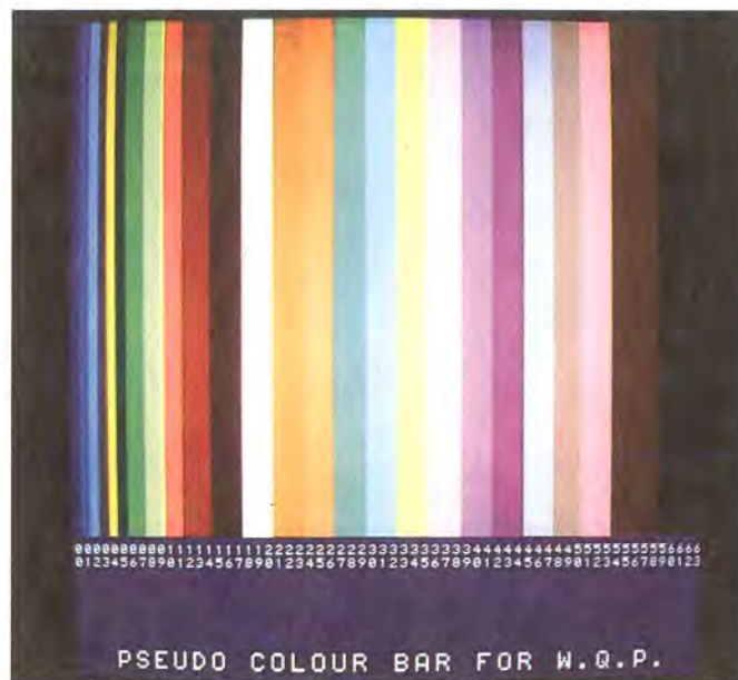
PLATE 3.1: COLOUR CODED BAR SHOWING THE FULL RANGE OF 0 - 255 REFLECTANCE VALUES DIVIDED INTO 25 COLOUR CLASSES
