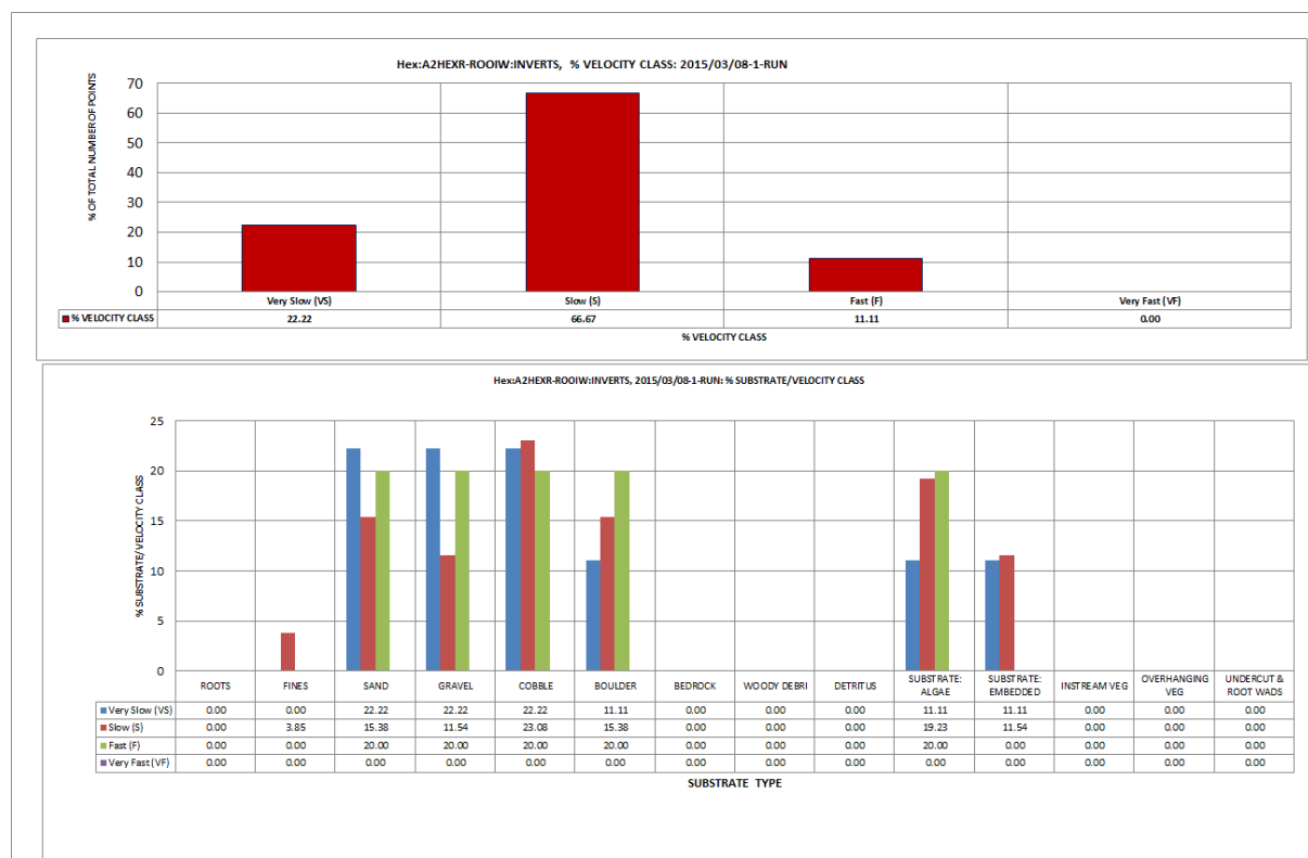
FIGURE 12-16. VELOCITY-DEPTH CLASSES AS A % OF ALL CROSS-SECTION POINTS (TOP GRAPH) AND % SUBSTRATE PRESENT PER VELOCITY-DEPTH CLASS (BOTTOM GRAPH), FOR MACROINVERTEBRATES AS AT MARCH 2015
