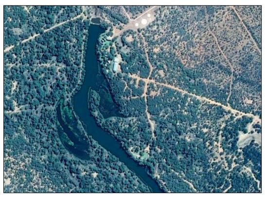
Figure 5-3: Illustration of inundation due to instream weir on the Matlabas River (Google Earth imagery, 2016)
