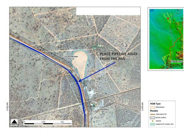
Figure 39. Pipeline placement on Leliesfontein to negate the impact on the wetland D3 5
