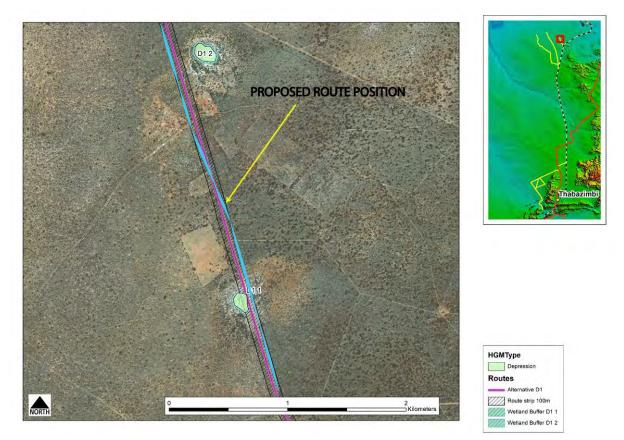
Figure 40. Pipeline placement on Enkeldraai and Taaiboshfontein to negate the impact on wetlands D1.1 and D1.2
