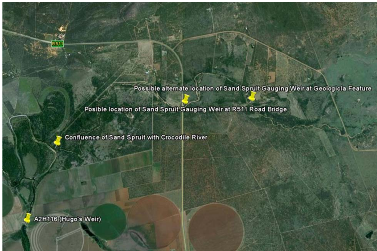
Figure 5-2: Plan View of Possible Gauging Weir Locations along Sandrivier
