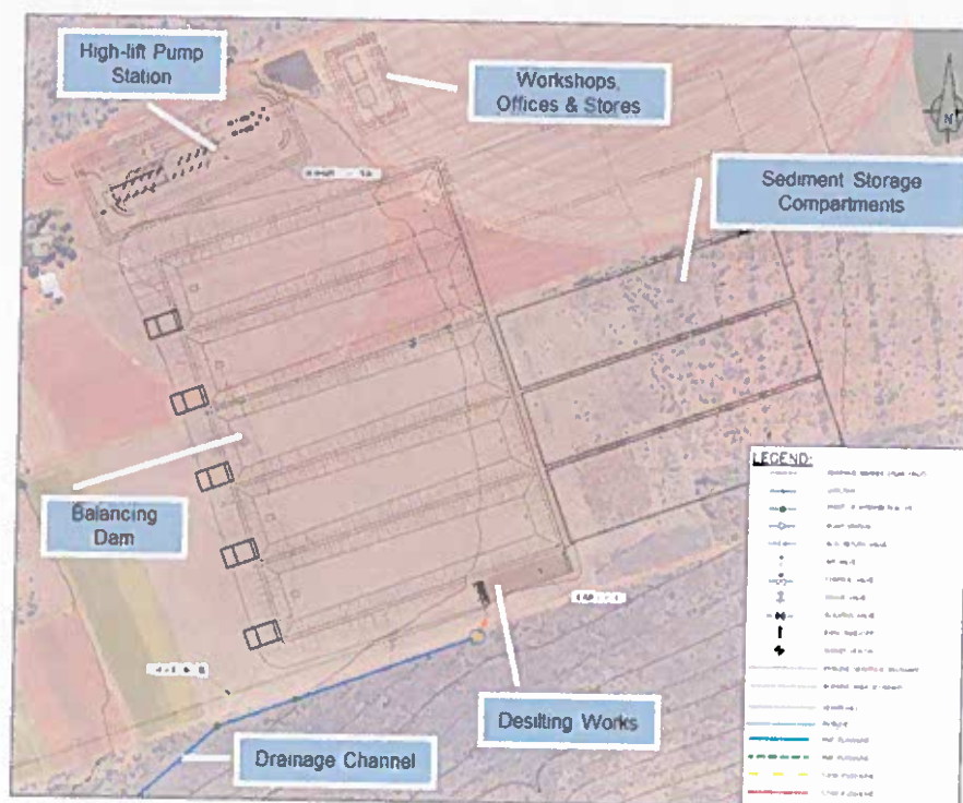
Figure 3: Balancing Dams, Desilting Works and High-lift Pump Station
