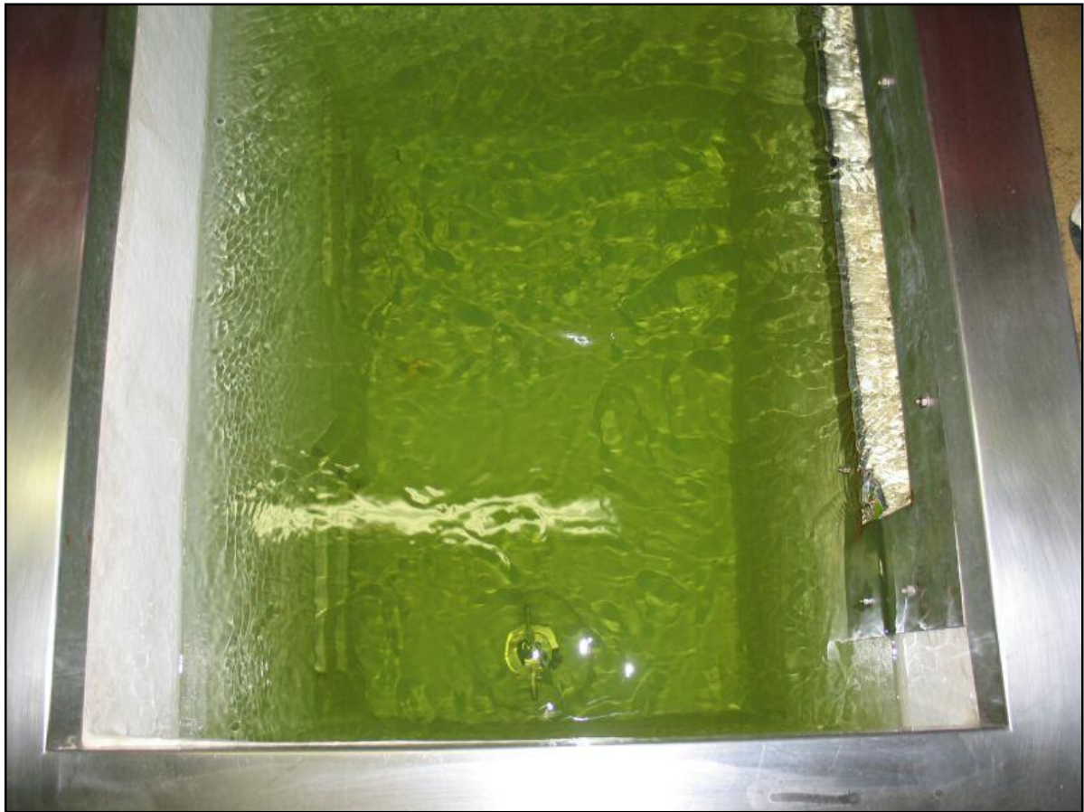
Figure 101: Final effluent water from Sedibeng Water purification plant (3/6/2006) – note the green colour of the water because of high residual algal concentrations (chlorophyll- a concentration >1 µg/ℓ)
