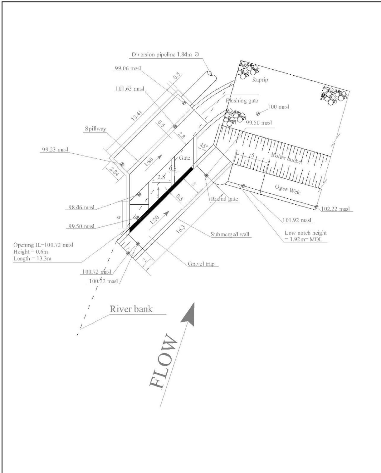
Figure 5.4 Typical layout of a 4 m<sup>3</sup>/s diversion weir on the Upper Wit River
