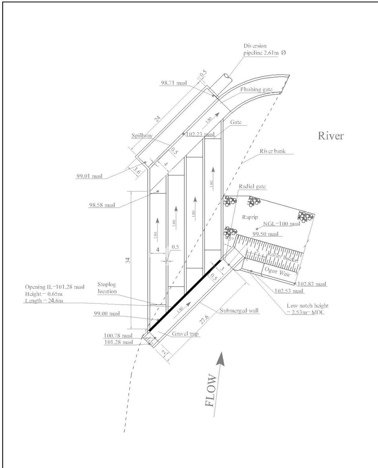
Figure 4.4 Typical layout of an 8 m<sup>3</sup>/s diversion weir at Michell's Pass
