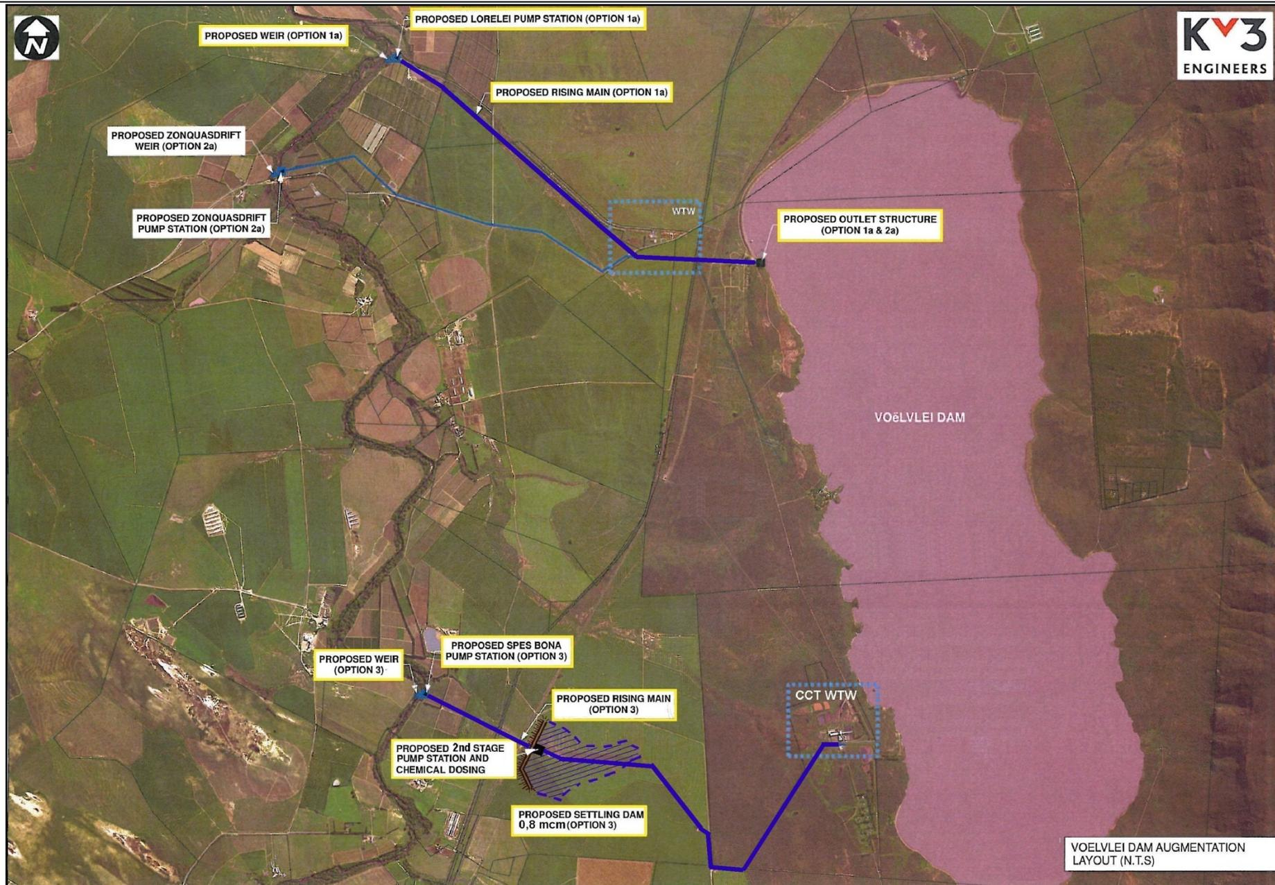
Figure 7.1 The proposed layout of the Voëlvlei Phase 1 options
