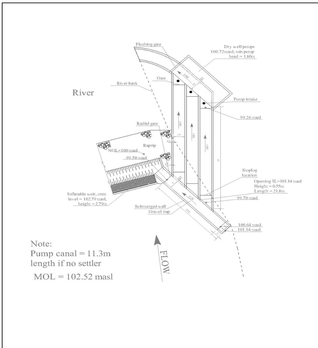
**Figure 7.3** Typical layout of a 6 m<sup>3</sup>/s diversion weir on the Berg River
