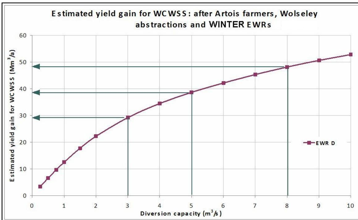
**Figure 4.5 Yield estimates for various diversion capacities at Michell’s Pass**
