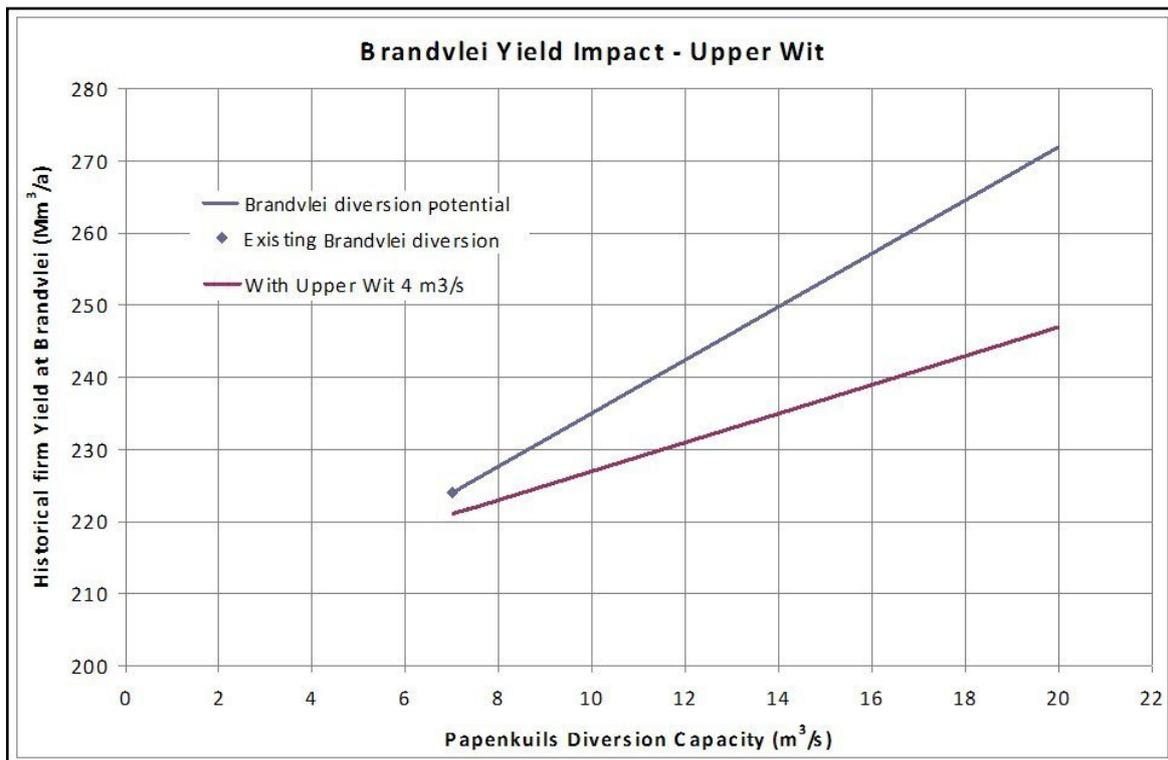
Figure 5.6 Pumping reinstatement for Brandvlei Dam (Upper Wit Scheme)
