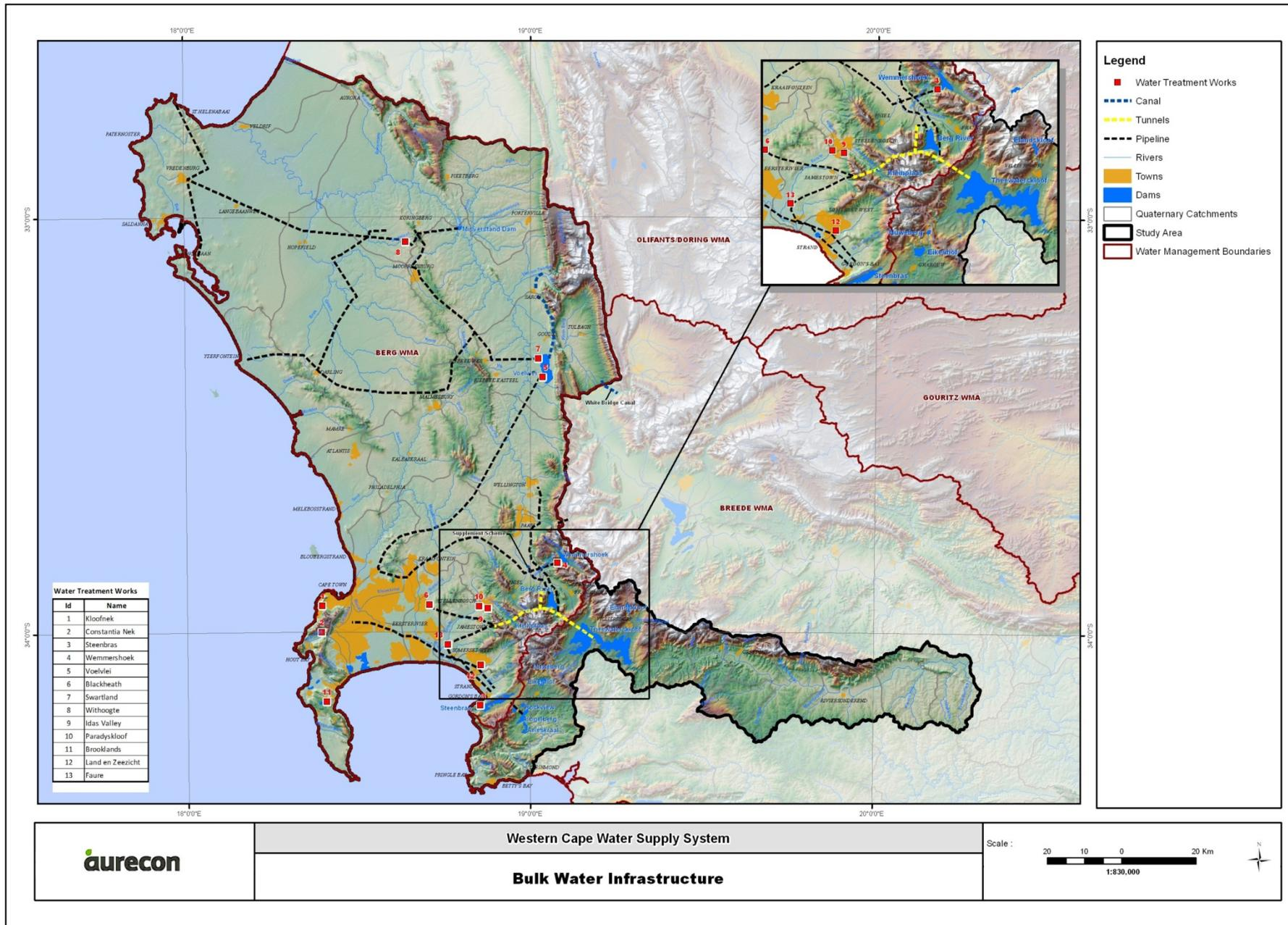
Figure 1.2 Layout of the WCWSS including Existing Infrastructure
