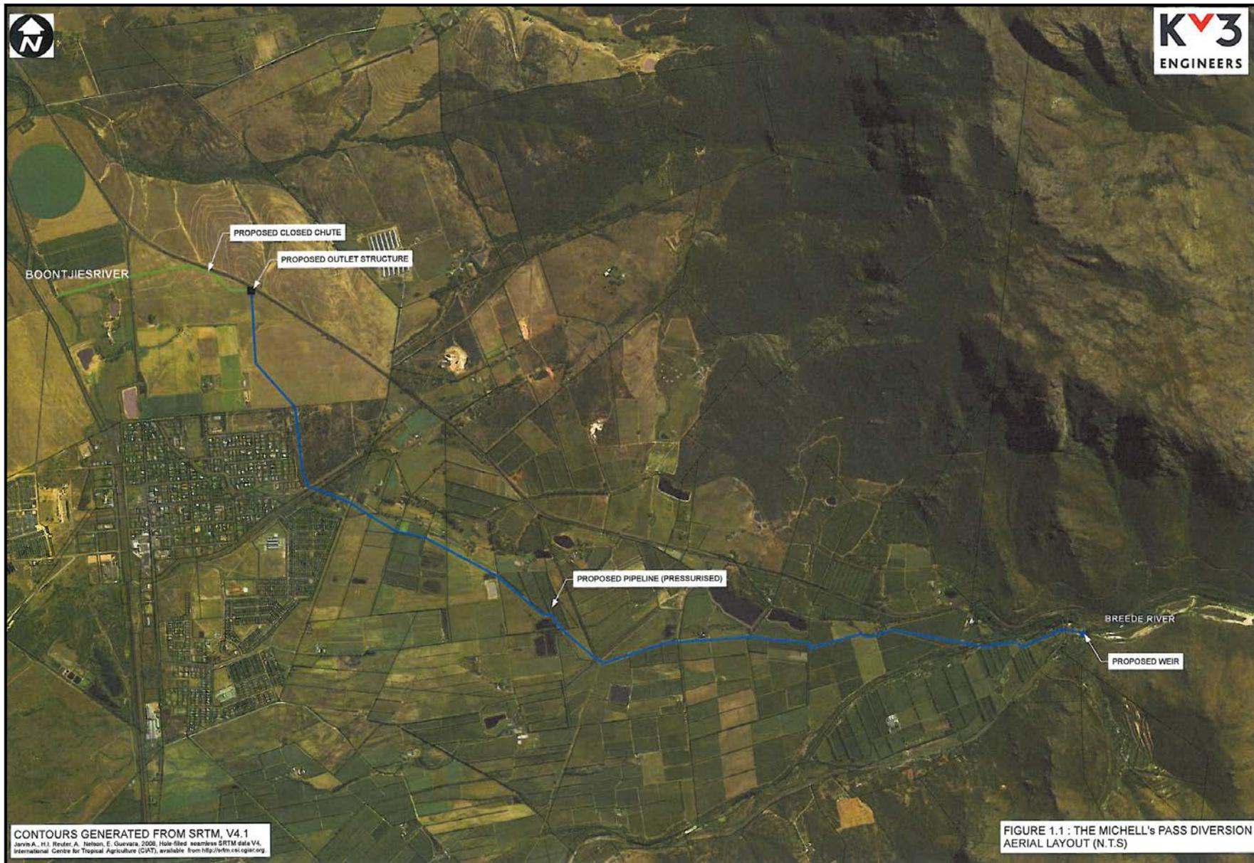
Figure 4.3 The proposed general layout of the Michell's Pass diversion scheme
