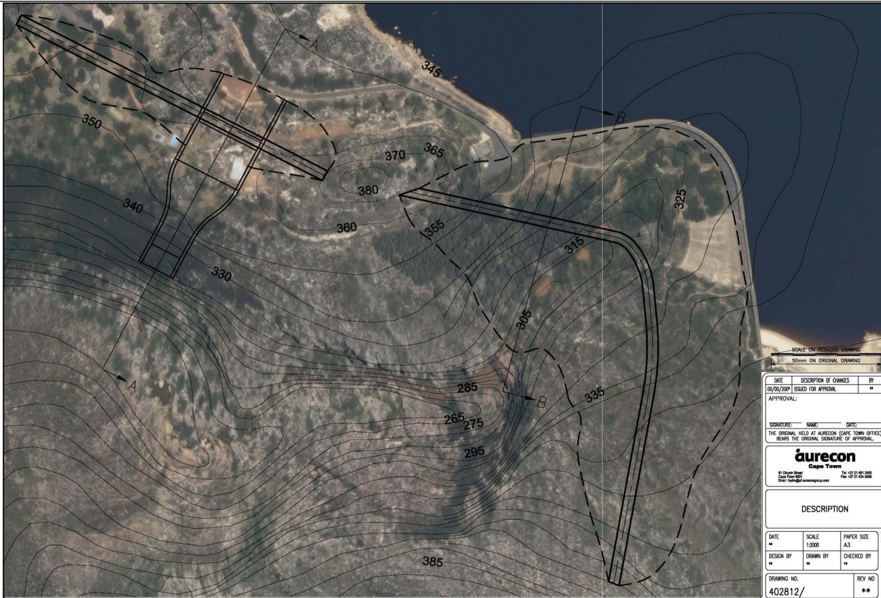
Figure 9.1 Plan Layout of Potential Rockfill Dam, Saddle Dam and Spillway
