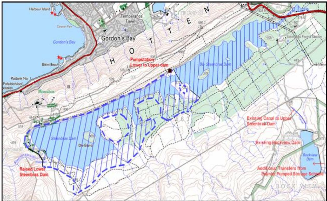
**Figure 9.3 The Full Supply Footprint Area of a Raised Lower Steenbras Dam**
