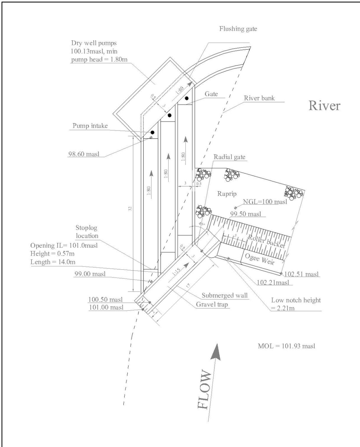
Figure 6.4 Typical layout of a 4 m<sup>3</sup>/s diversion weir on the Molenaars River
