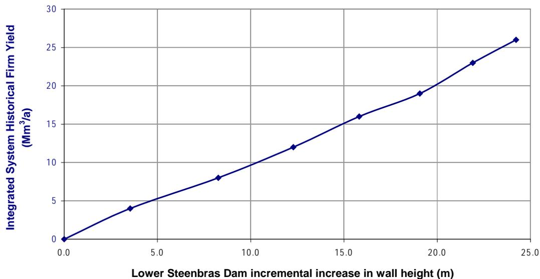
"i:\hydro\400820\wrym\ib8\out\Steenbras Scenarios.xls" sheet "Plot wall heights Lower Integ"
