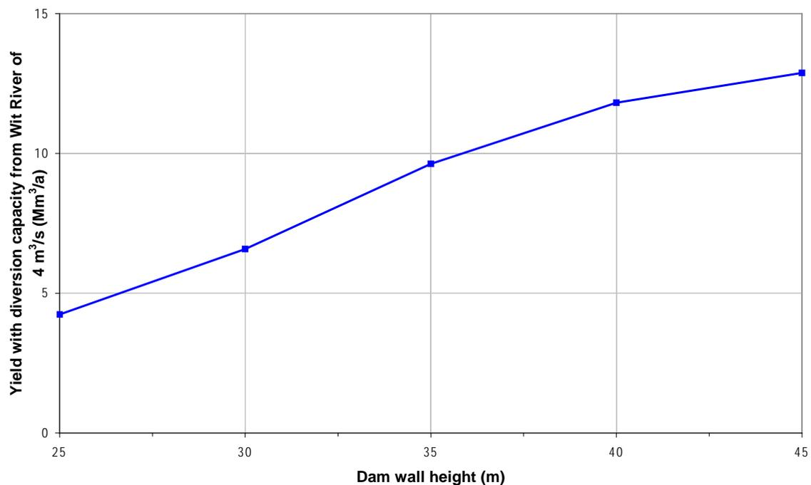
**Figure 5 : Historical firm yield for given wall heights of the proposed Wit River diversion into Doolhof Dam scheme for a diversion capacity off the Wit River of 4 m<sup>3</sup>/s**
