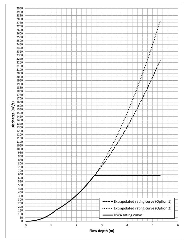
Figure 4.2: Flow gauging station U1H005 rating curve
