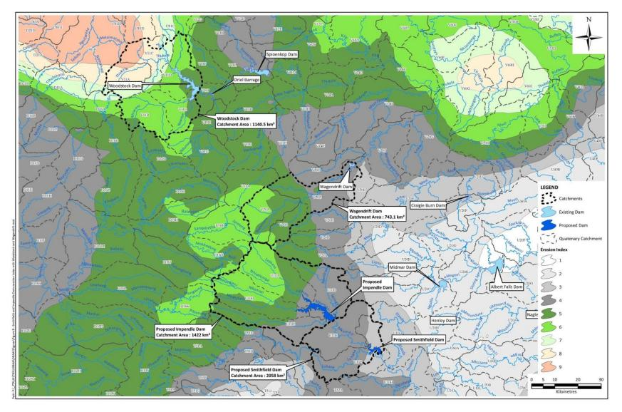
Figure 5.4:Impendle, Smithfield, Woodstock and Wagendrift Dam Catchments Comparative Erosion Index (2010<br/>Sediment Yield Prediction)
