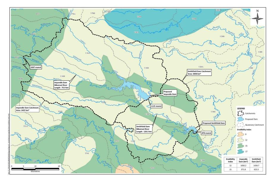
Figure 5.1: Impendle and Smithfield Dam Catchments Erodibility Index (1992 Sediment Yield Map)
