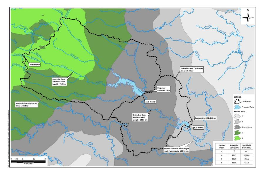
Figure 5.3: Impendle and Smithfield Dam Catchments Erosion Index (2010 Sediment Yield Prediction)
