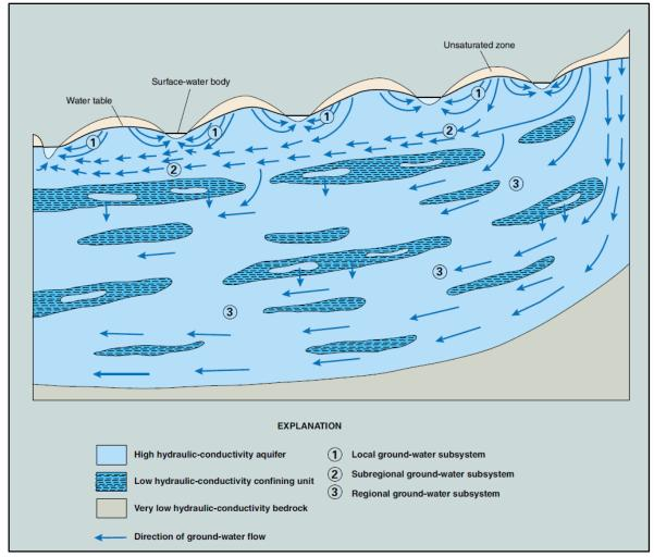
Figure 6: Groundwater flow systems (USGS, 1999)
