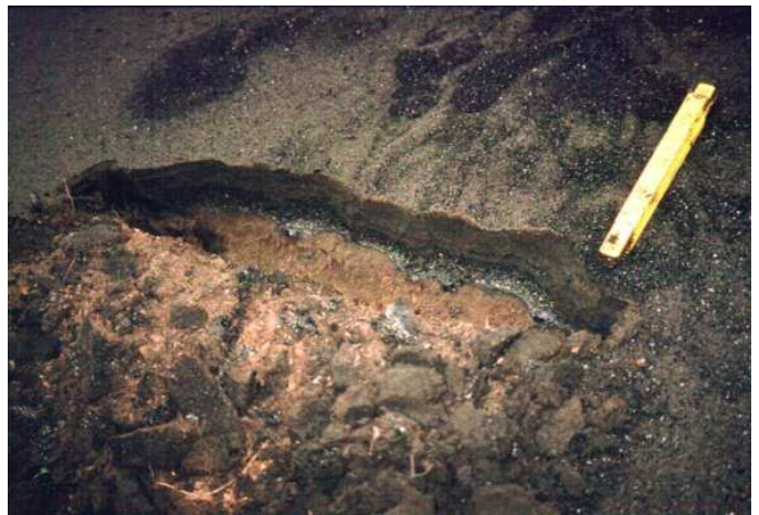
Soil profile showing the wettable surface layer (darker wet soil) above the water repellent layer (dry soil), 31 May 2000, four months after the fire. Alien vegetation occurred on the site. The yellow ruler is 20 cm long.
