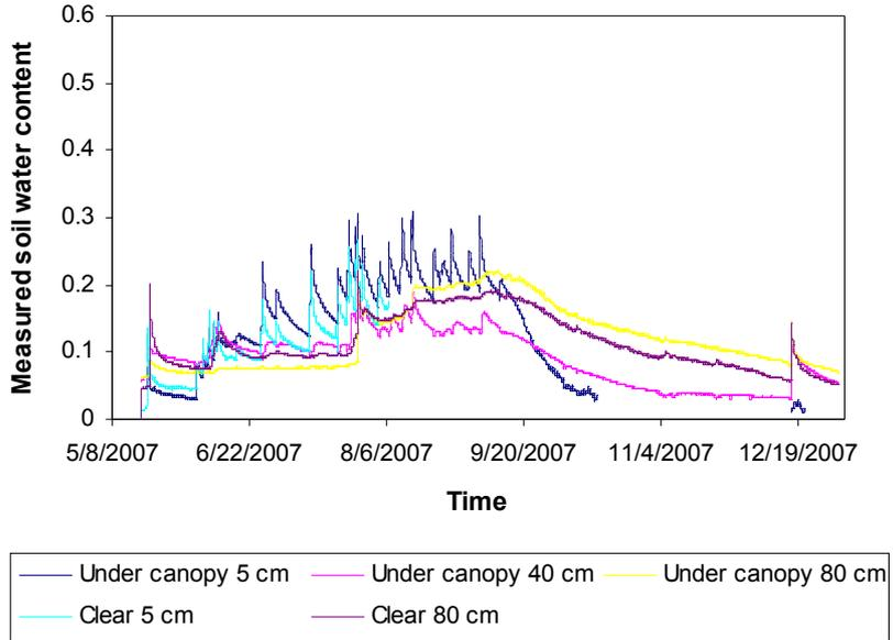
Figure 13: Volumetric soil water contents measured with Echo-sensors at different soil depths and positions in the Uncleared treatment at Riverlands.
