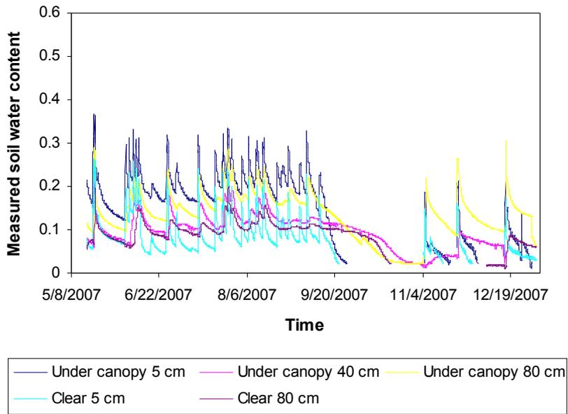
Figure 14: Volumetric soil water contents measured with Echo-sensors at different soil depths and positions in the Cleared treatment at Riverlands.
