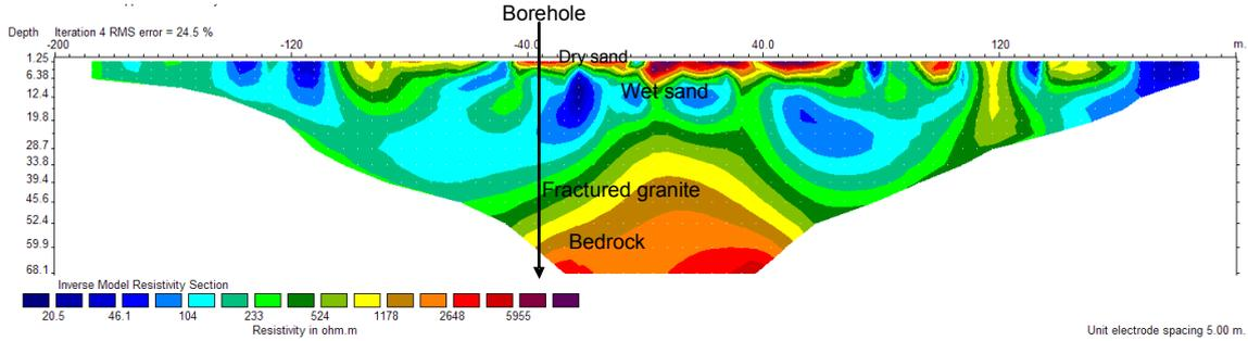
Figure 4: Deep resistivity survey profile next to the existing 120 m deep borehole.
